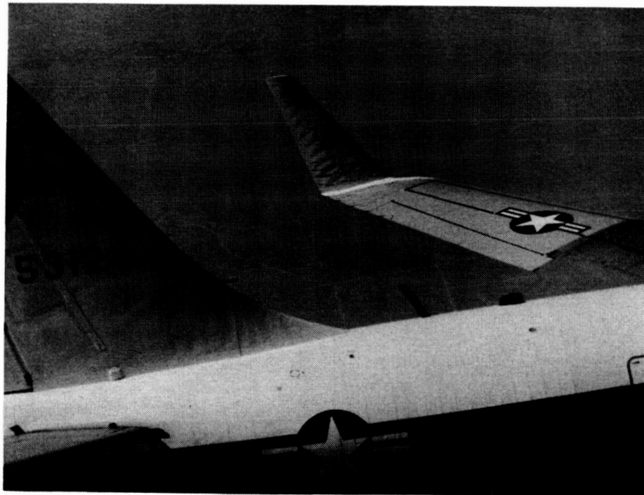
Figure 8. - Winglet in flight with skin "pillowing"
