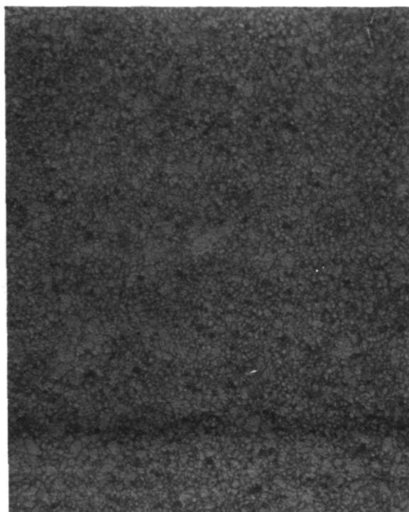
Figure 18. - Optical micrograph of undoped hot pressed \text{Al}_2\text{O}_3 sample annealed at 1630^\circ\text{C} for 10 hr. (160X).
