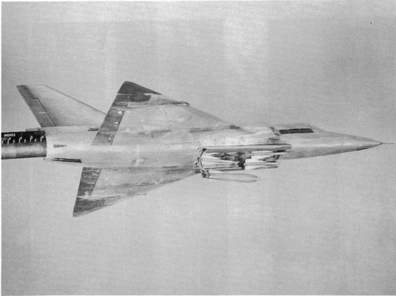
Figure 7.- Convair F-106 wind tunnel model showing stores.
