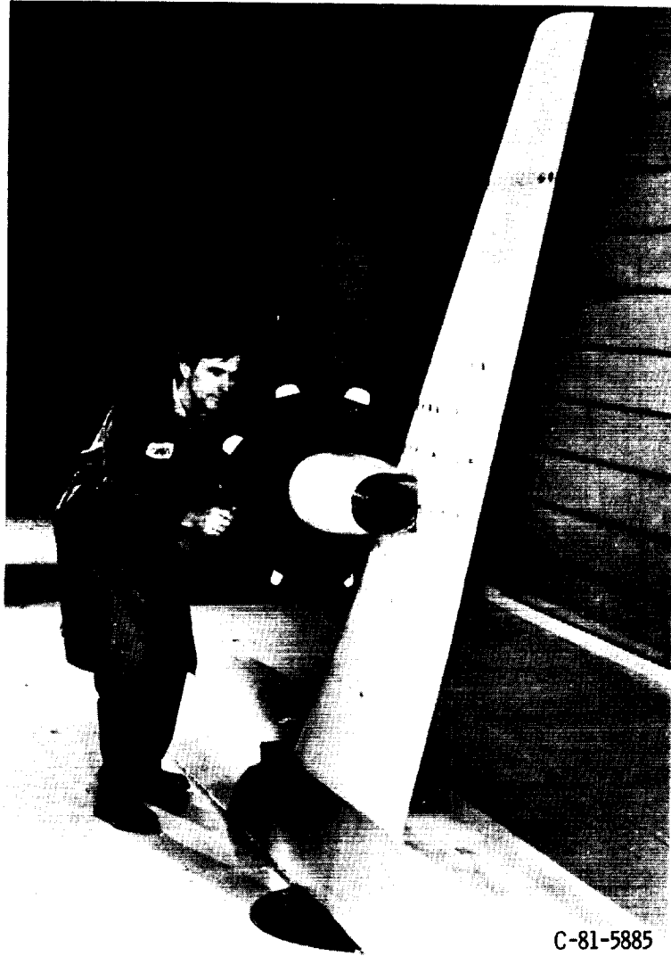
Figure 29. - Photograph of the SR-2C (8-bladed, 0^{\circ} sweep) propeller installed on the semi-span aircraft model in the Ames 14-foot transonic wind tunnel.
