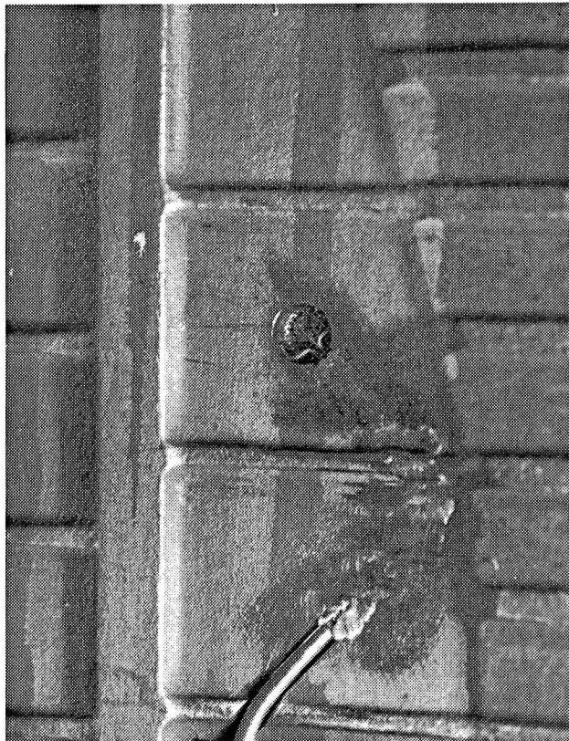
Figure 5.2-7 Gardon Gauge Sensor - Three Conductor Wire Installed
