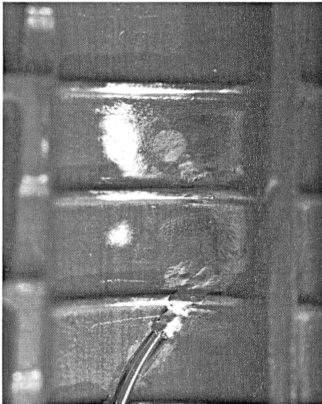
Figure 5.2-8 Gardon Gauge Sensor - Ceramic Cement in Place
