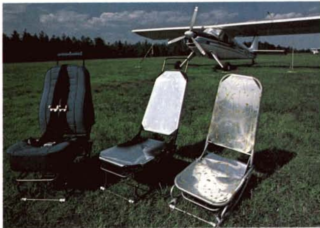
Shown above are JAARS safety seats with and without the foam pad and fabric covering.
