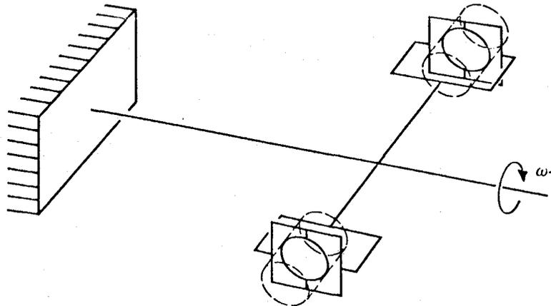
*To investigate otolith responses to fractional accelerations up to 1.25g along any arbitrary anatomical axis.*
