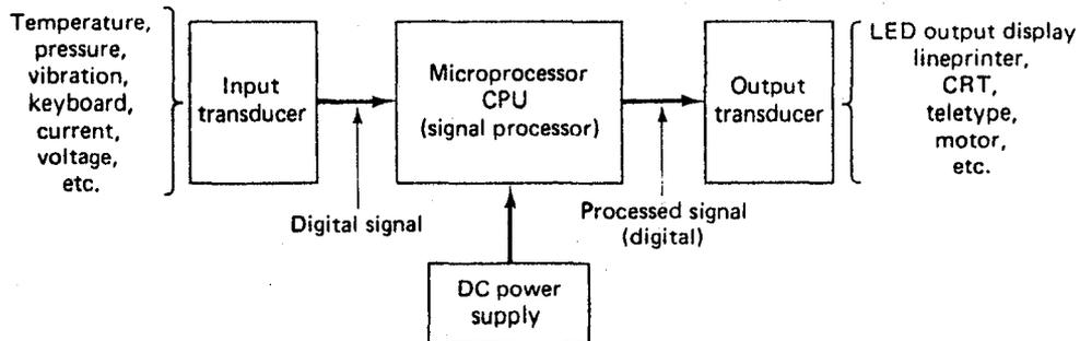
Figure 4.- Functional organization typical of most microprocessor systems.
