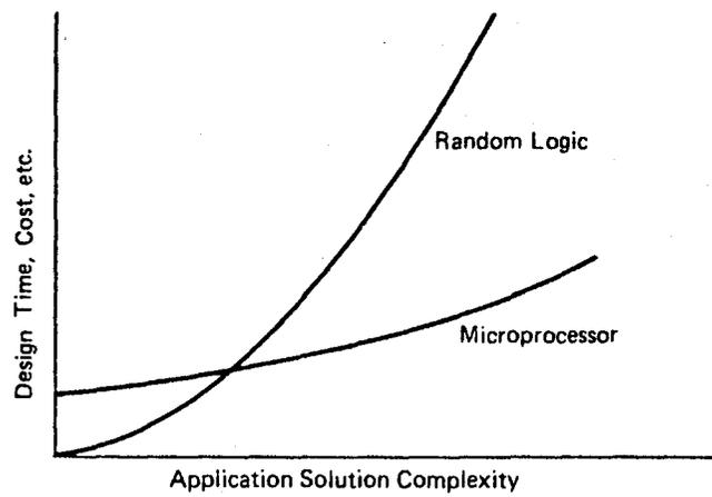
Figure 1.- Cost trends of random logic versus microprocessors.
