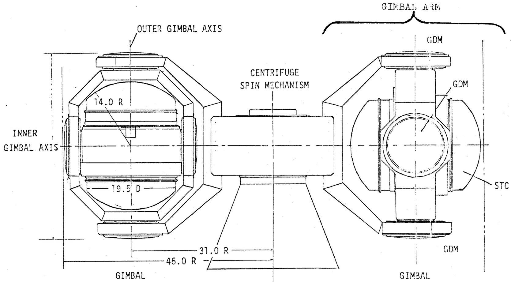
Figure 2.- Plan view of VRF ground centrifuge configuration.
