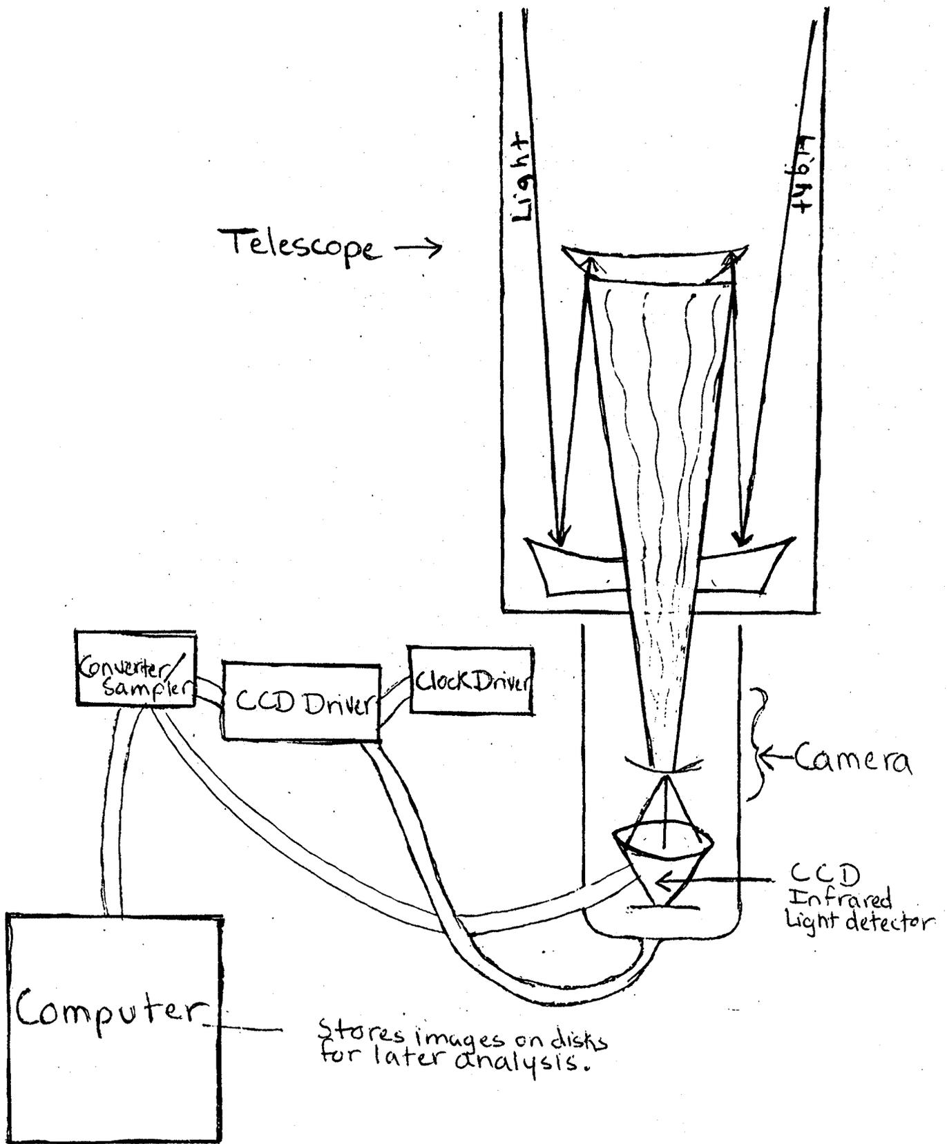
Figure 1.- Operation of the 10 μm infrared array camera.
