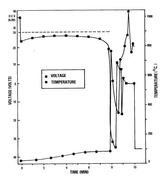
Figure 1. Voltage and temperature data for the forced discharge of a battery at 21 amperes.
