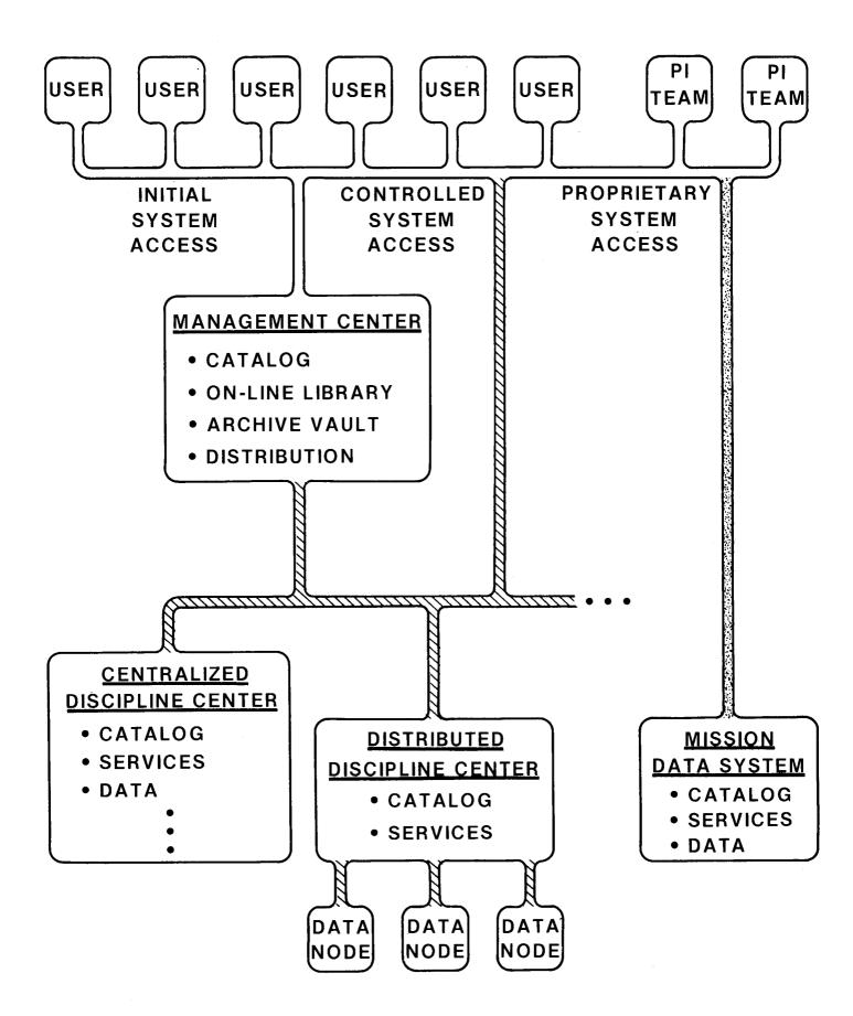
FIGURE 4.1 PRELIMINARY PDS FUNCTIONAL CONFIGURATION
