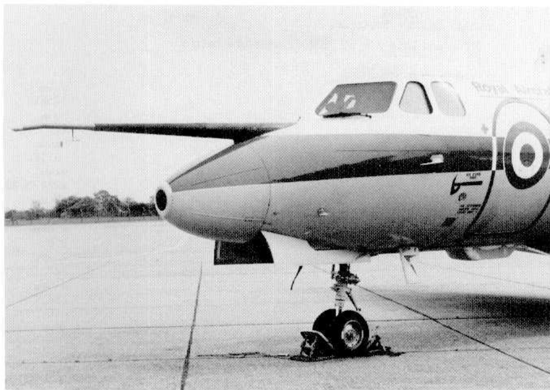
Fig. 5 The HS125 aircraft showing the nose cone and 20 cm diameter germanium window. See also fig. 8.
