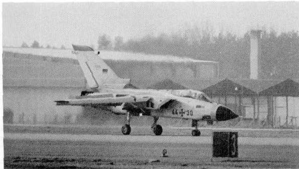
FIG. 1 TORNADO MULTI ROLE COMBAT AIRCRAFT IN MAX DRY T/R DECELERATION AFTER LANDING
