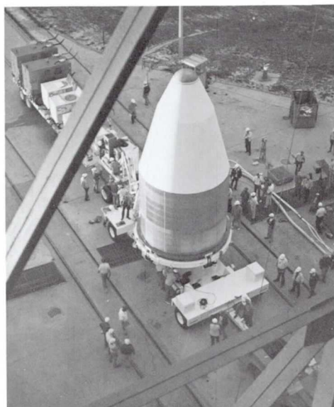
Viking orbiter 1, top left, is mated to Viking lander 1 at Kennedy Space Center on 8 March 1975. Above, technicians lower the launch shroud over the spacecraft on 27 March. At left, the shrouded orbiter and lander move toward 31 March mating with the Titan IIIE launch vehicle, for more tests.
