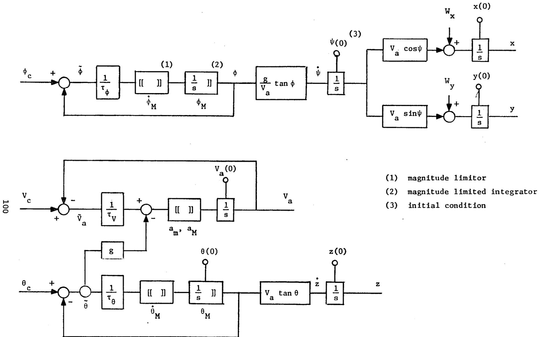
Figure 26. Simplified Command-Response Based Point Mass Aircraft Dynamic Model
