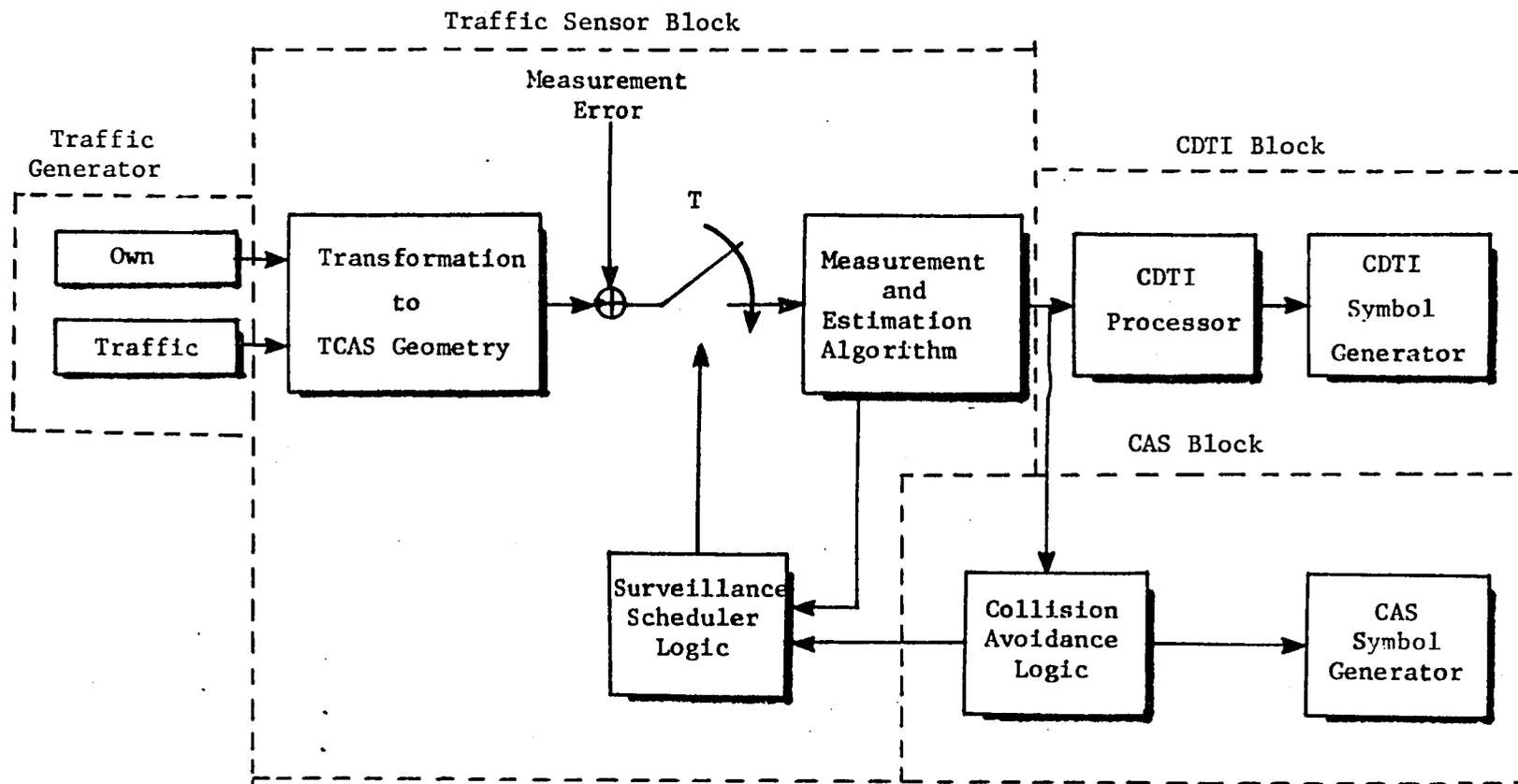
Figure 9. Enhanced BX TCAS II/CDTI Sensor Model Block Diagram
