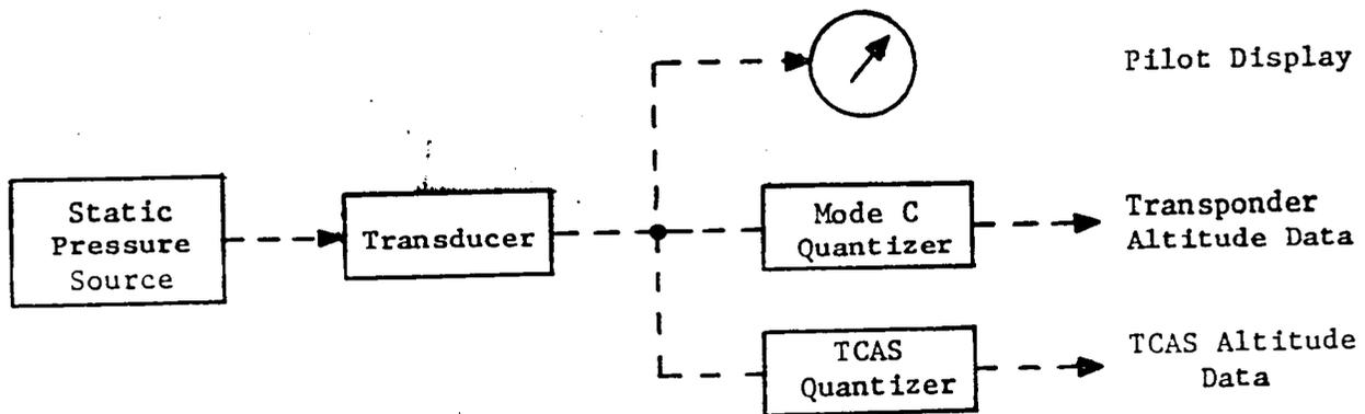
Figure 4. Schematic Diagram of Altitude Measurement Process.
