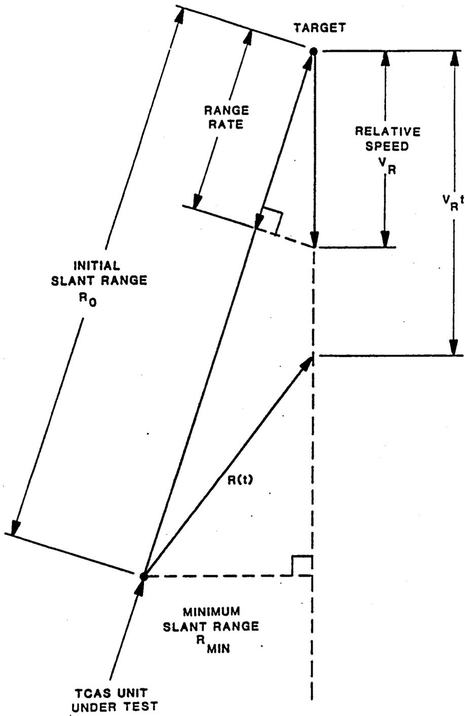
Figure 32. Definitions of Variables Associates with the Linear Movements of Targets in the Range Dimension
