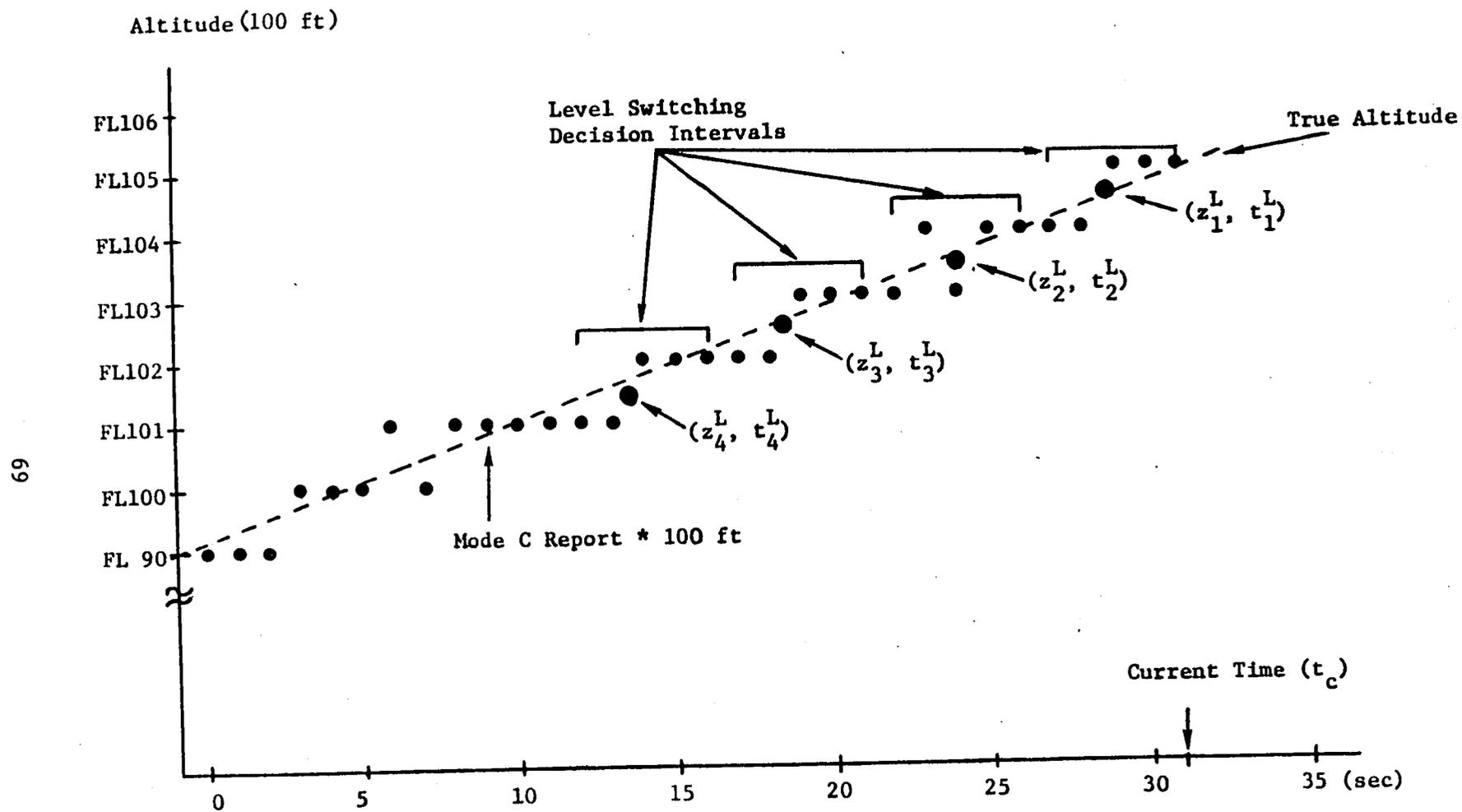
Figure 15. Illustration of Level Switching Times and Altitude Measurements
