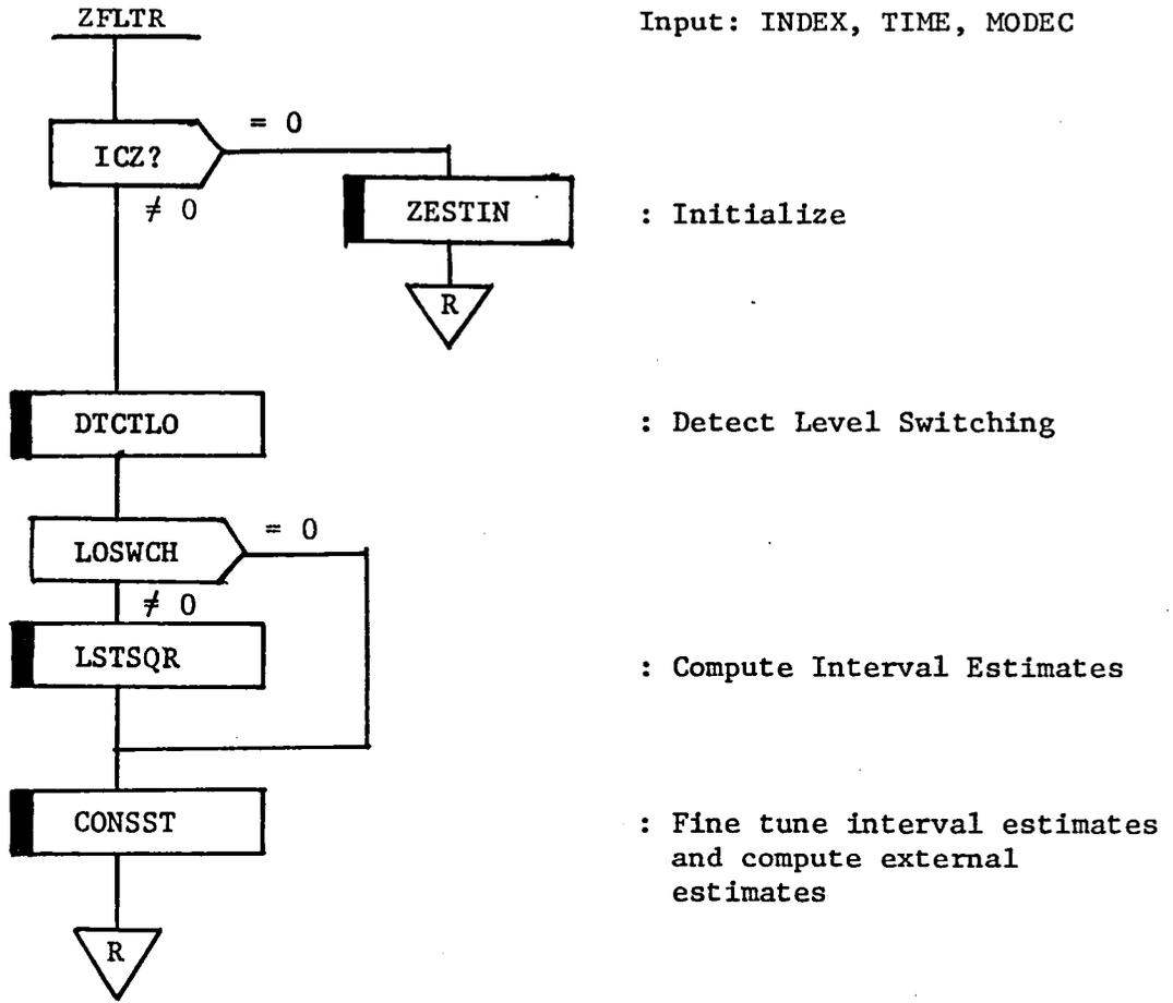
Figure 14. Vertical Tracker Algorithm Macro Flow Chart
