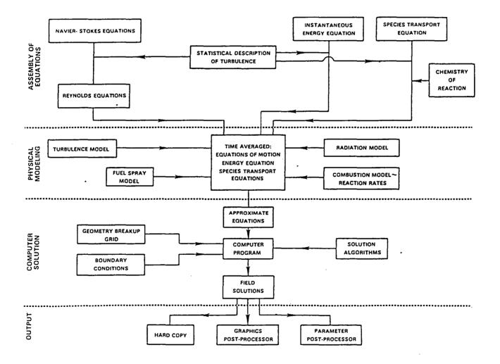
Figure 1 Flow Diagram of Calculation Procedure
