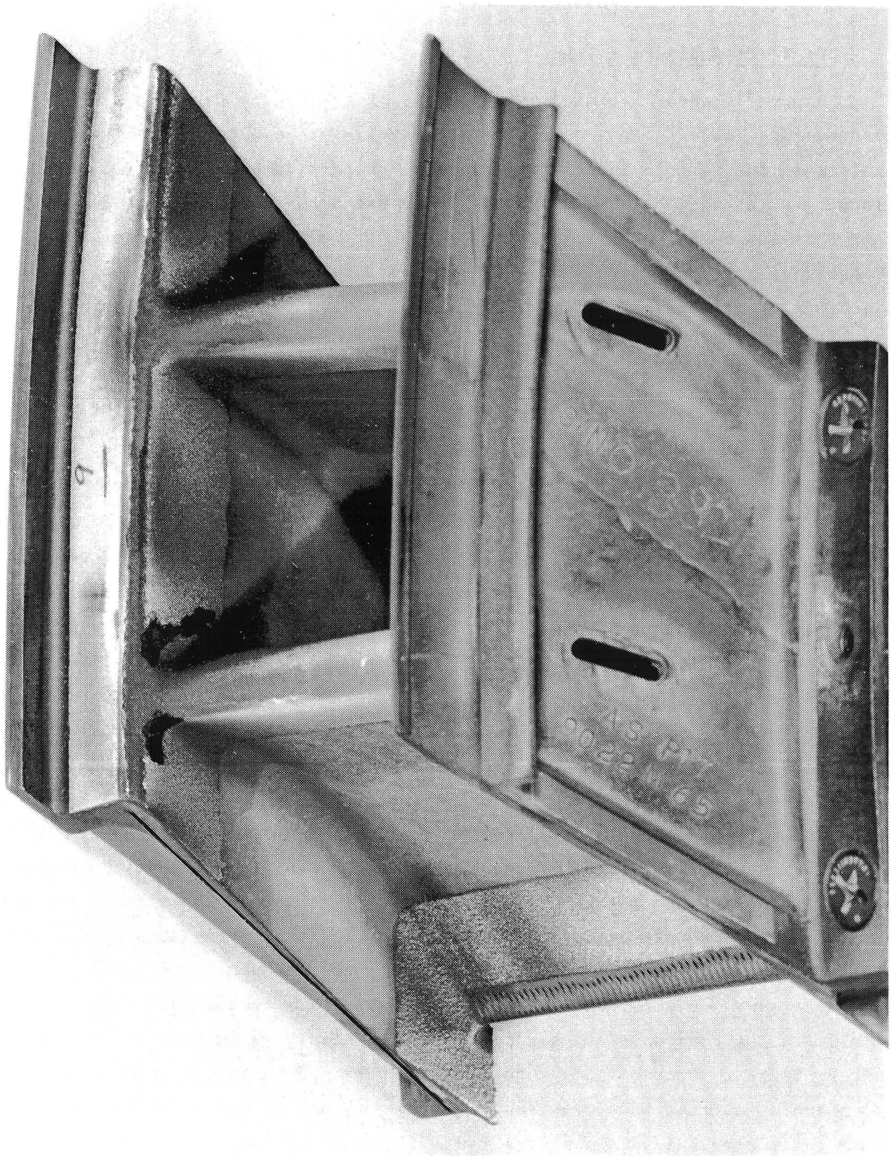
Figure 70. TBC CF6-50 Stage 2 Vane after 1000 Cycles.
