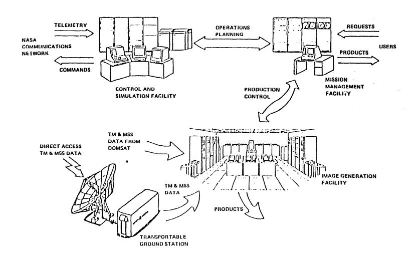
Figure 1 Landsat - 4/D' Ground Segment
