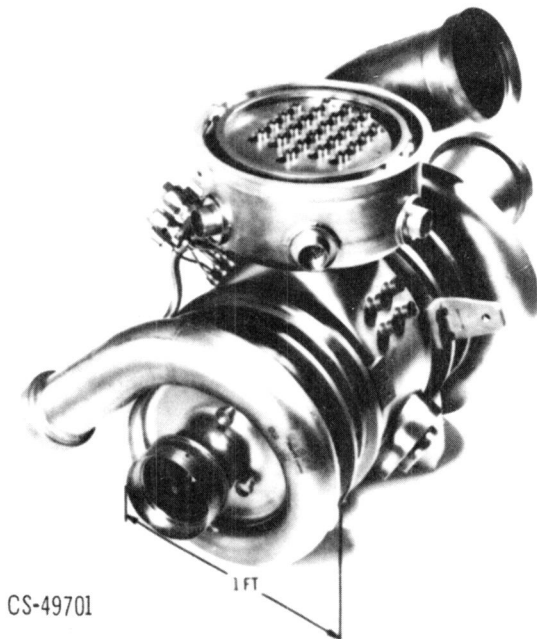
Figure 11. - Brayton rotating unit.
