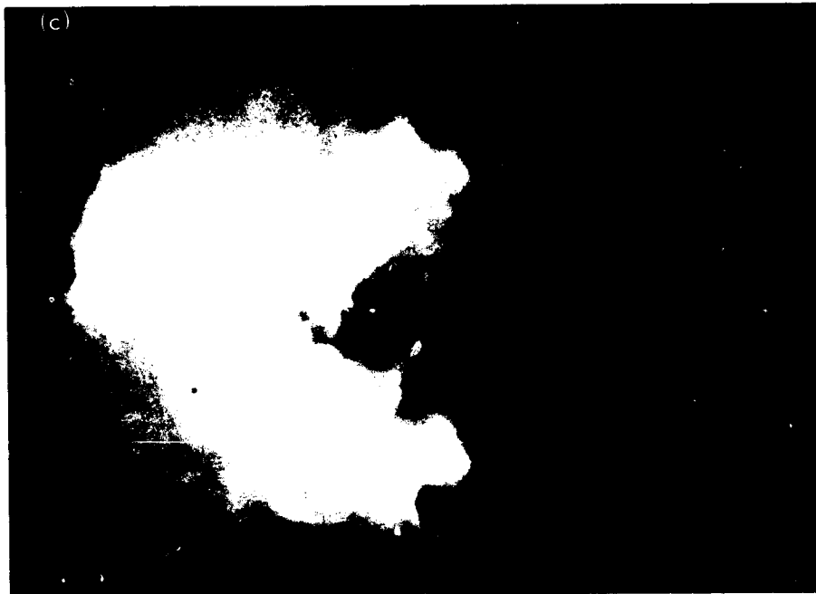
Figure 44. Halon flow test of the multicone nozzle at: (c) 4 ms
