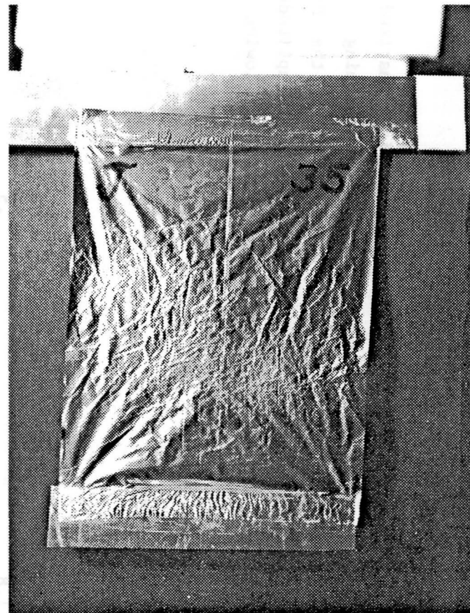
Figure 4.6 Tedlar tensioned to 0.22 \text{ MN/m}^2 (32.5 psi)
