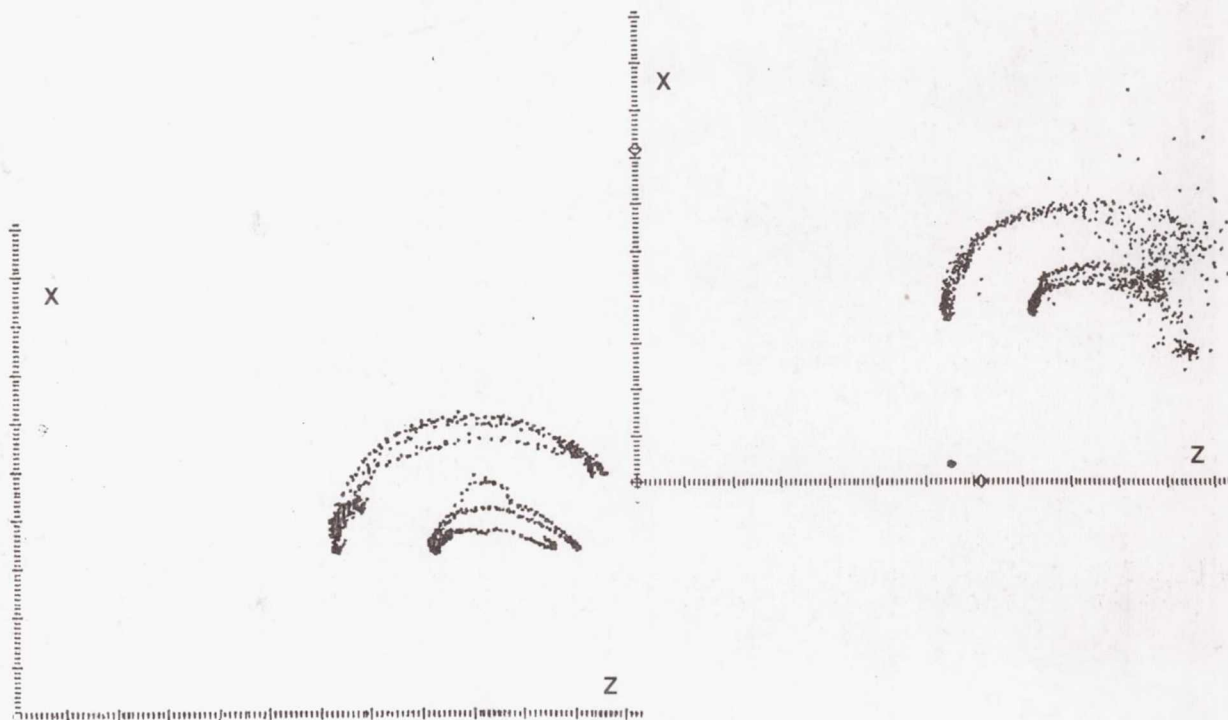
FIGURE 3.- SHOULDER ROTATION ARCS IN TWO PROTOTYPE SUITS. IRED'S WERE ATTACHED TO THE UPPER ARM AND ELBOW.
