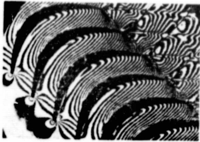
Figure 4.24. Measurement of turbine blade by Mach Sender interference.
