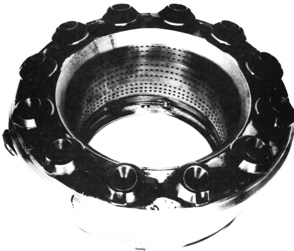
Figure 6B. Dilution Flow Impingement Cooled Combustor
