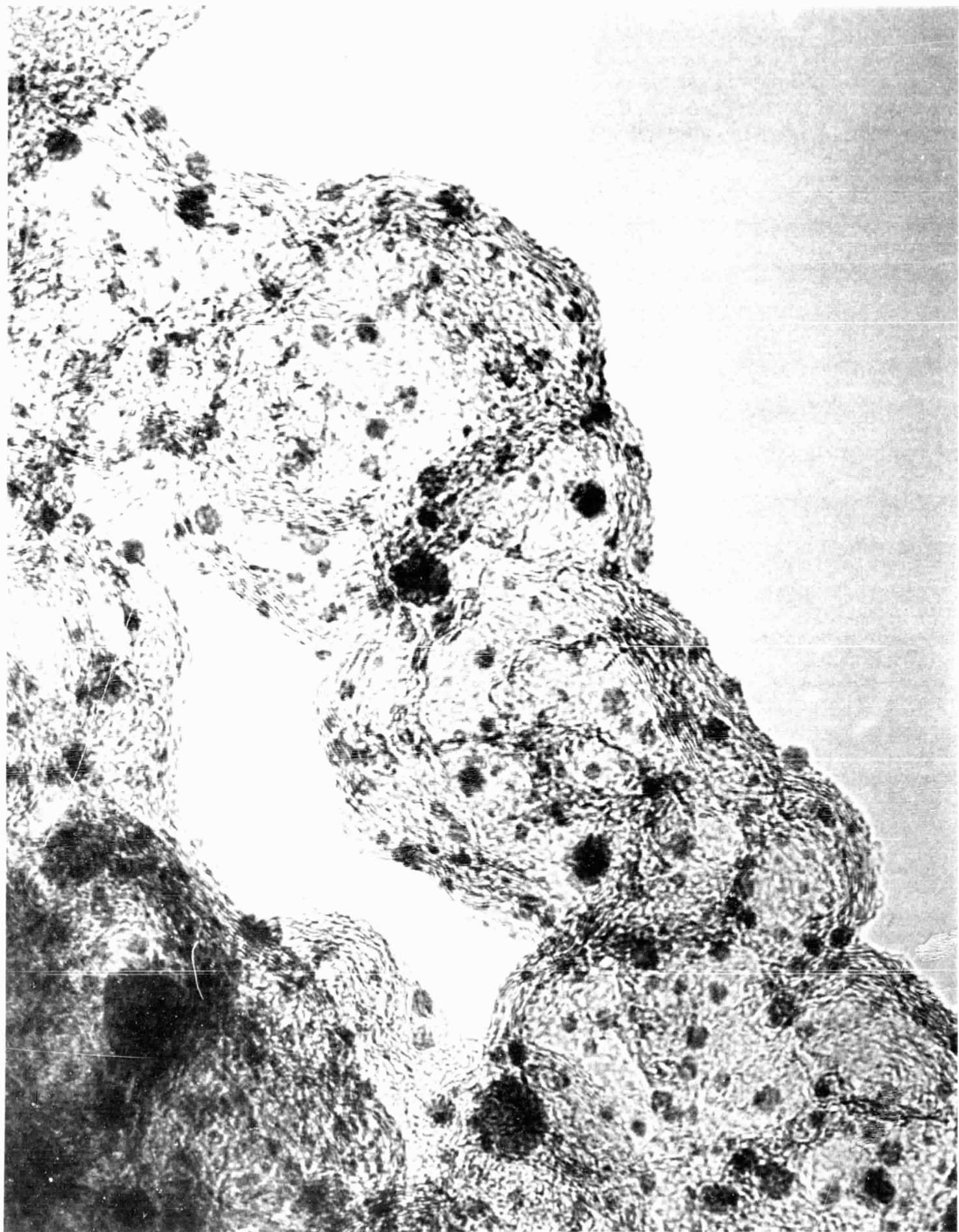
Figure 37. EC 123 4 w/o Pt-Pd (50 a/o Pd) on Consel 1. 2,035,000X mag.
