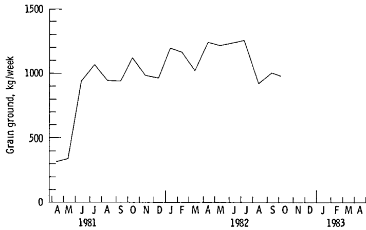
Figure 4 - Flour production with Tangaye photovoltaic system
