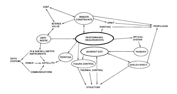
To produce a technology development plan for LDR, it was decided to undertake the System Concept and Technology Definition Studies. The purpose of the studies is to understand the interaction of the various systems of LDR and to understand the impact of the systems issues on the total system.
