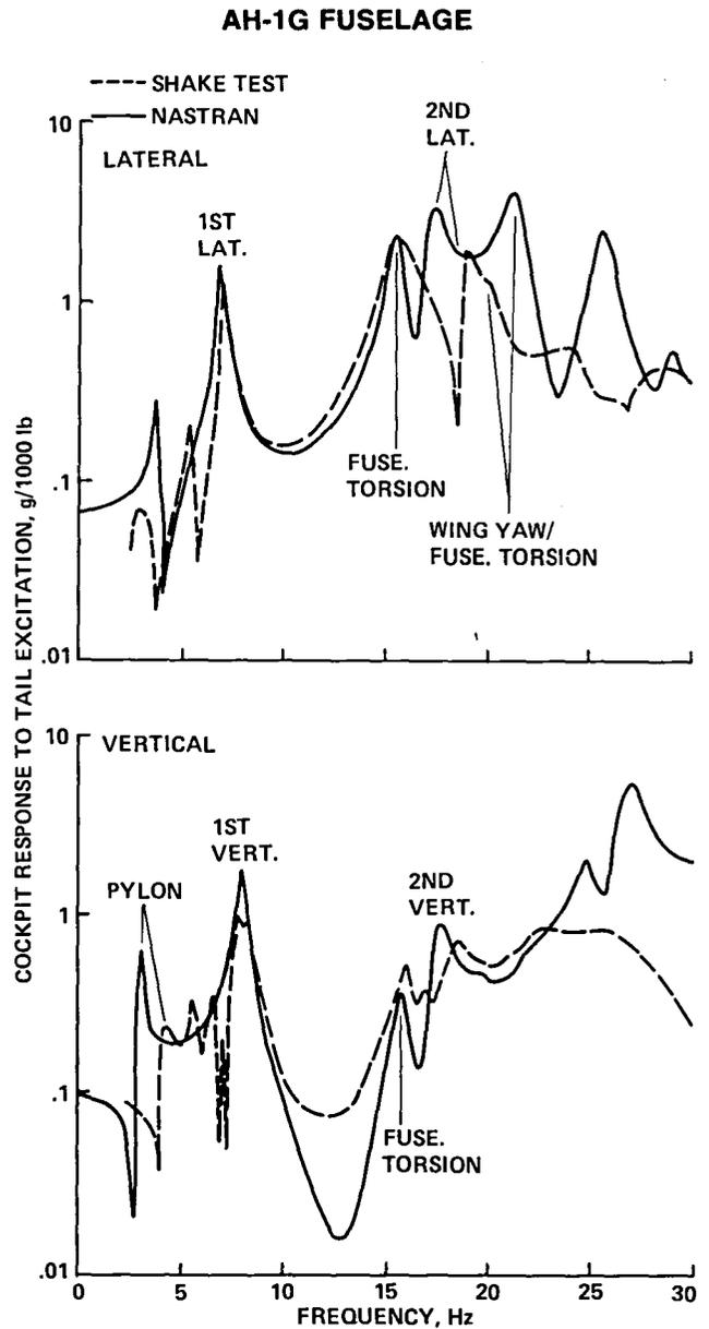
Fig. 66. Airframe structural dynamics (Ref. 65).
