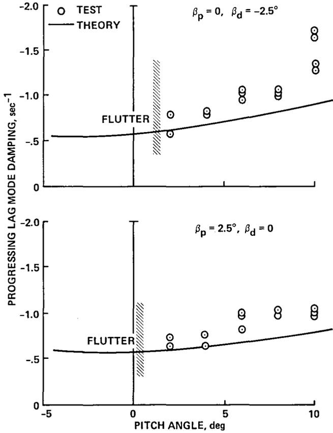
Fig. 44. Bearingless rotor stability (Ref. 42).
