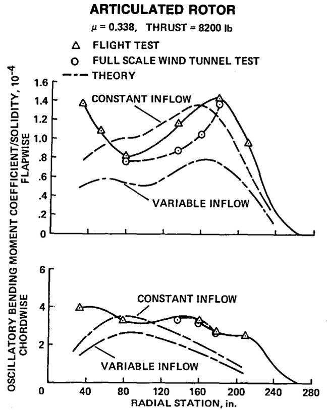
Fig. 56. Articulated rotor blade loads (Ref. 62).
