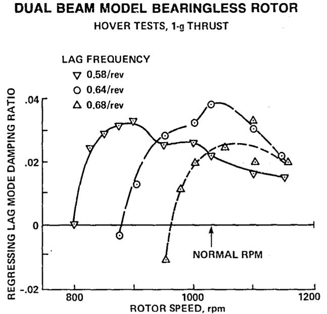
Fig. 111. Measured model bearingless rotor stability (Ref. 116).
