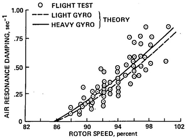
Fig. 104. XH-51A bearingless helicopter stability (Ref. 112).
