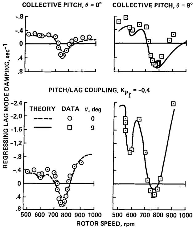
Fig. 47. Hingeless rotor ground resonance stability (Ref. 47).
