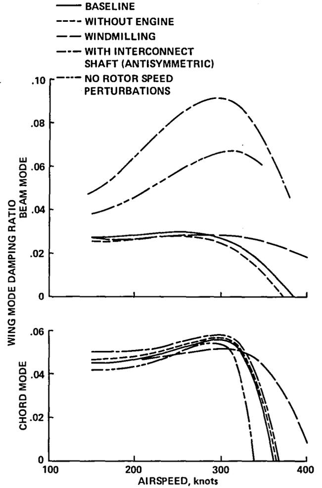
Fig. 130. Calculated tilting prop-rotor aircraft whirl flutter stability.
