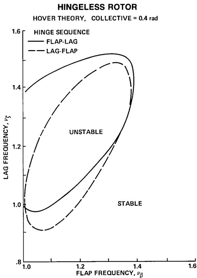
Fig. 15. Calculated flap-lag stability (Ref. 16).
