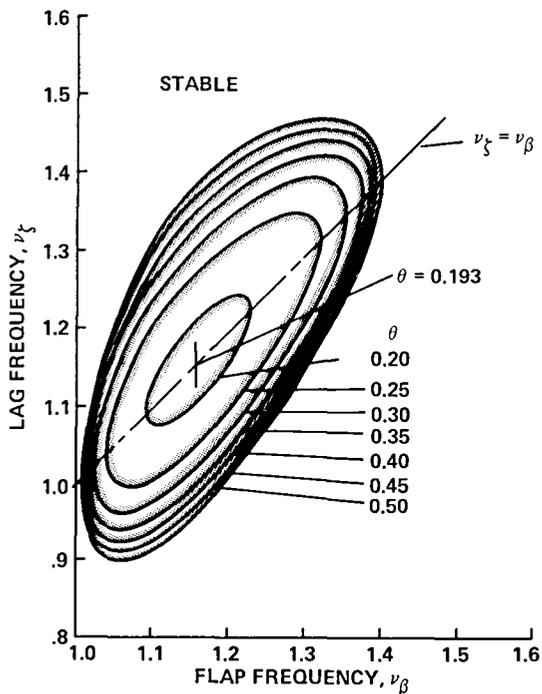
Fig. 3. Calculated flap-lag stability boundaries (Ref. 8).
