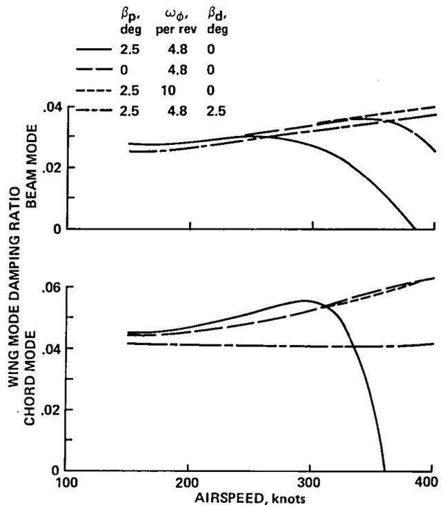
Fig. 127. Calculated tilting prop-rotor aircraft whirl flutter stability.
