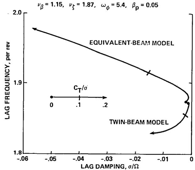
Fig. 46. Calculated bearingless rotor root locus (Ref. 44).
