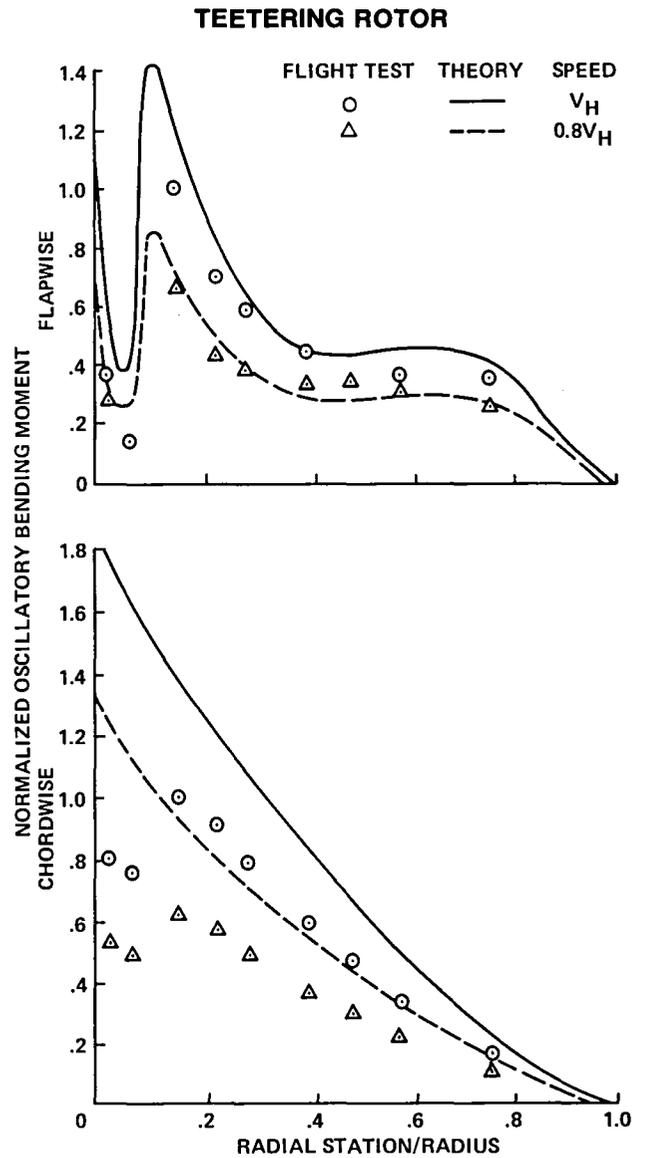
Fig. 58. Teetering rotor blade loads (Ref. 61).
