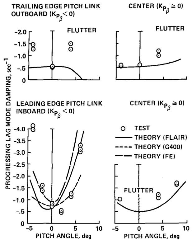
Fig. 43. Bearingless rotor stability (Ref. 42).
