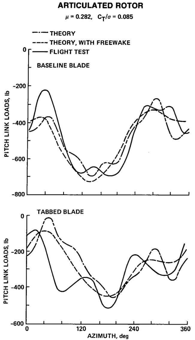
Fig. 64. Articulated rotor blade loads (Ref. 51).
