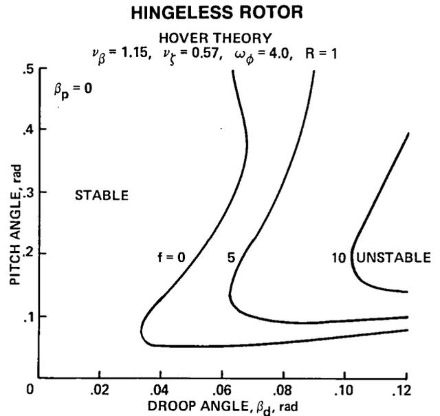
Fig. 26. Calculated pitch-flap-lag-torsion stability boundaries (Ref. 26).
