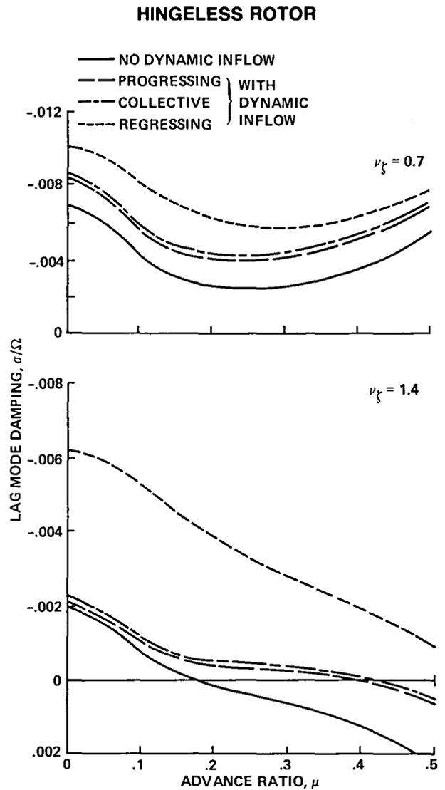
Fig. 82. Calculated flap-lag stability with dynamic inflow (Ref. 86).
