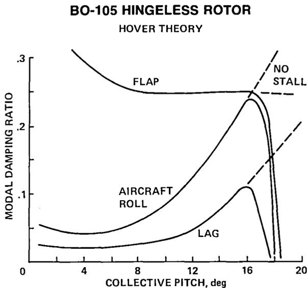
Fig. 11. Calculated flap-lag instability produced by stall (Ref. 12).
