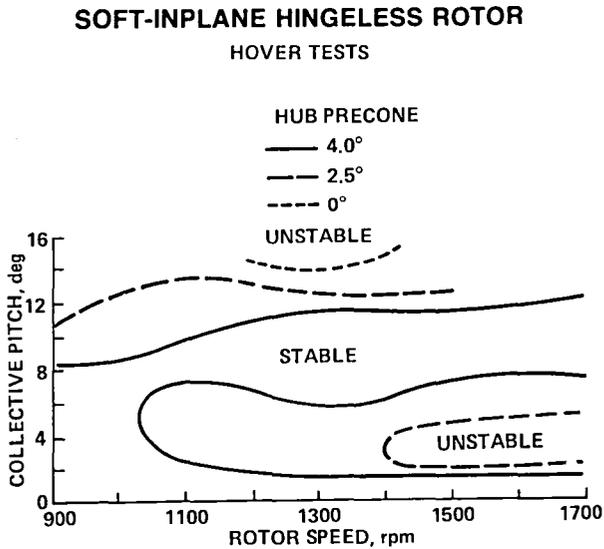
Fig. 7. Measured soft-inplane hingeless rotor stability boundaries (Ref. 10).
