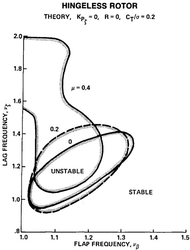
Fig. 33. Calculated flap-lag stability boundaries (Ref. 31).
