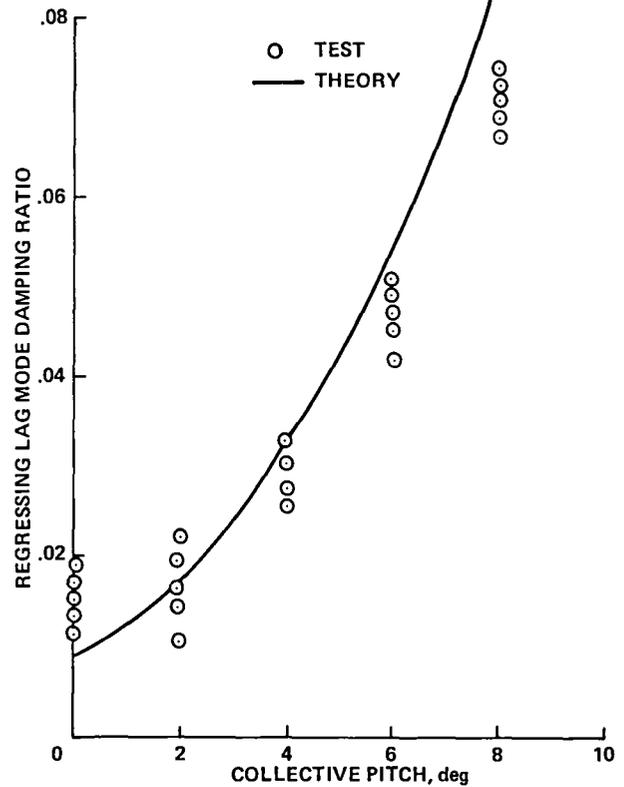
Fig. 40. Bearingless Main Rotor (BMR) stability (Ref. 40).
