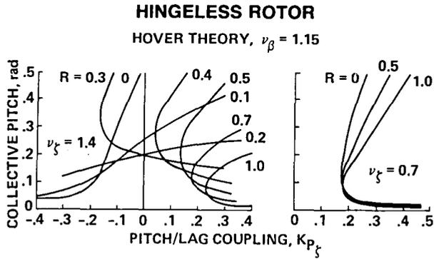
Fig. 5. Calculated flap-lag stability boundaries (Ref. 8).
