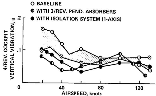
Fig. 103. Measured BK-117 helicopter vibration (Ref. 110).
