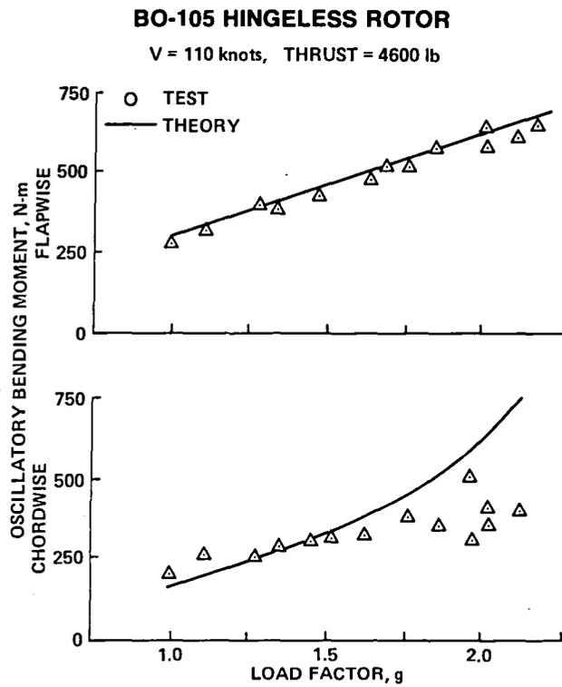
Fig. 55. Hingeless rotor blade loads (Ref. 57).
