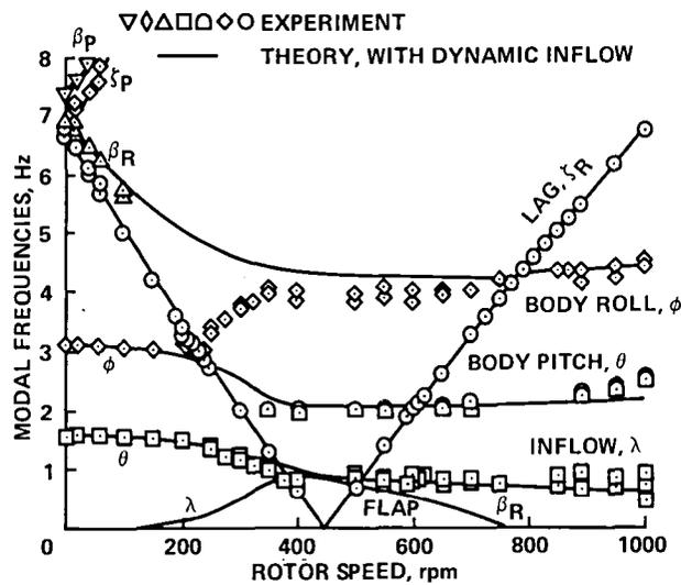
Fig. 85. Ground resonance stability with dynamic inflow (Ref. 80).
