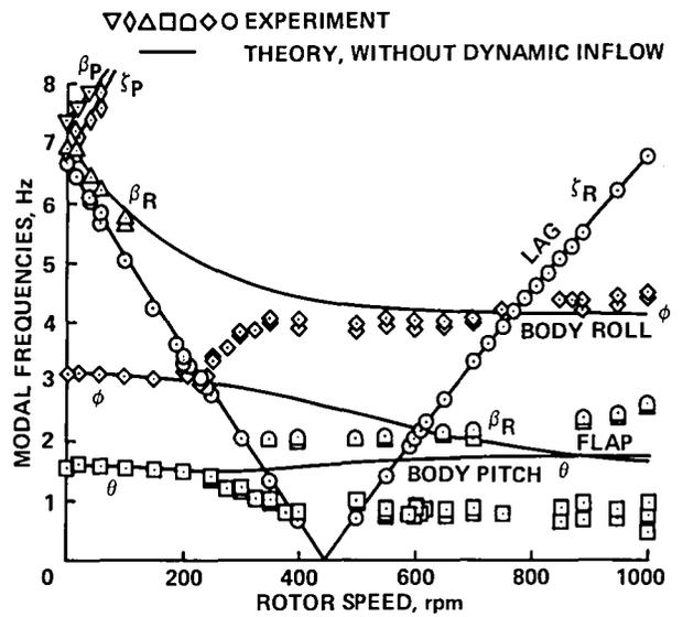
Fig. 84. Ground resonance stability with dynamic inflow (Ref. 80).
