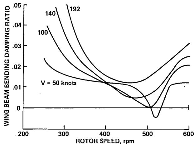
Fig. 128. Calculated tilting prop-rotor aircraft air resonance stability.
