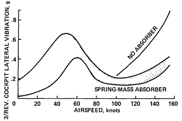
Fig. 98. Measured ABC helicopter vibration (Ref. 106).
