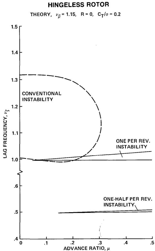
Fig. 36. Calculated flap-lag stability boundaries (Ref. 31).
