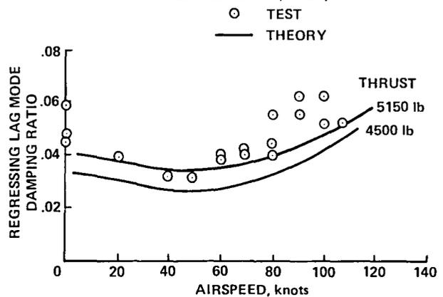
Fig. 41. Bearingless Main Rotor (BMR) stability (Ref. 40).
