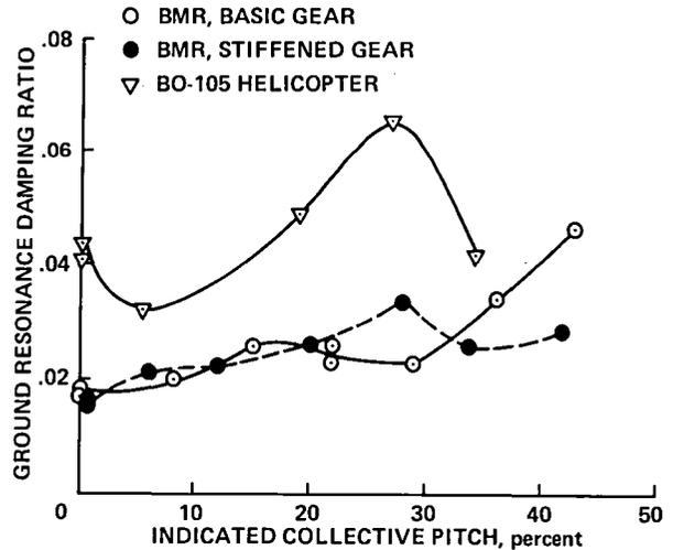
Fig. 107. Measured BMR bearingless helicopter stability (Ref. 113).
