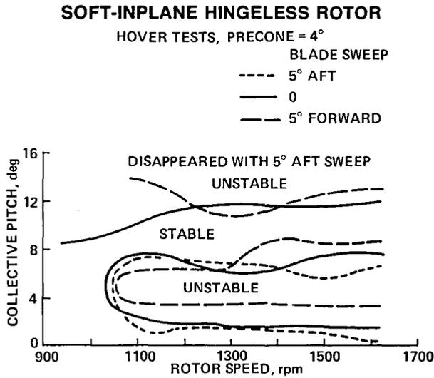
Fig. 9. Measured soft-inplane hingeless rotor stability boundaries (Ref. 10).
