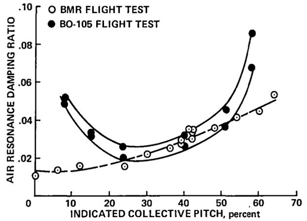
Fig. 105. Measured BMR bearingless helicopter stability (Ref. 113).
