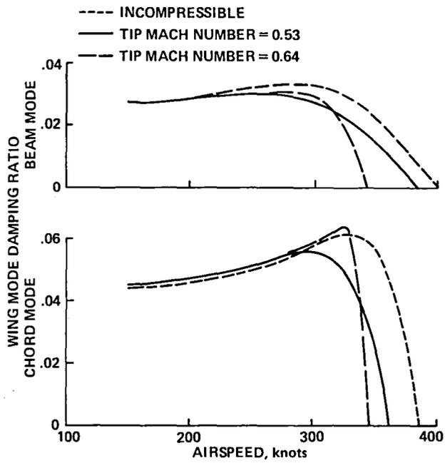
Fig. 129. Calculated tilting prop-rotor aircraft whirl flutter stability.
