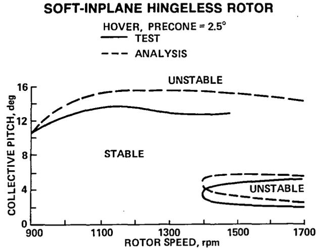
Fig. 6. Soft-inplane hingeless rotor stability boundaries (Ref. 10).
