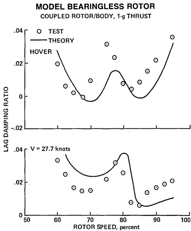
Fig. 115. Small scale Model 680 bearingless rotor stability (Ref. 119).
