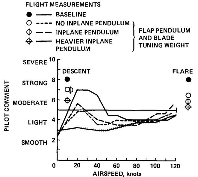
Fig. 74. Measured hingeless rotor vibration reduction (Ref. 68).
