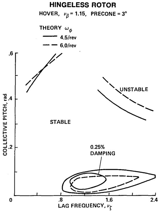
Fig. 28. Calculated flap-lag-torsion stability boundaries (Ref. 27).
