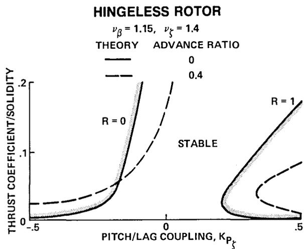
Fig. 35. Calculated flap-lag stability boundaries (Ref. 31).
