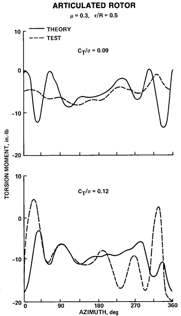
Fig. 62. Articulated rotor blade loads (Ref. 60).
