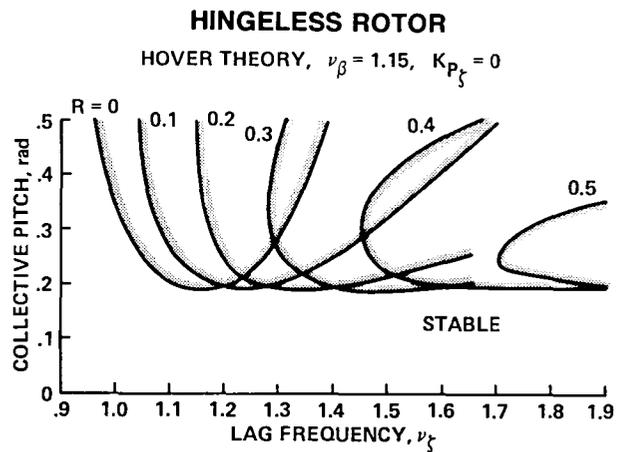
Fig. 4. Calculated flap-lag stability boundaries (Ref. 8).
