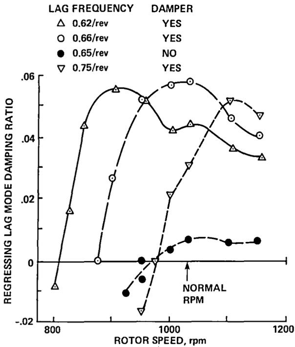
Fig. 112. Measured model bearingless rotor stability (Ref. 116).
