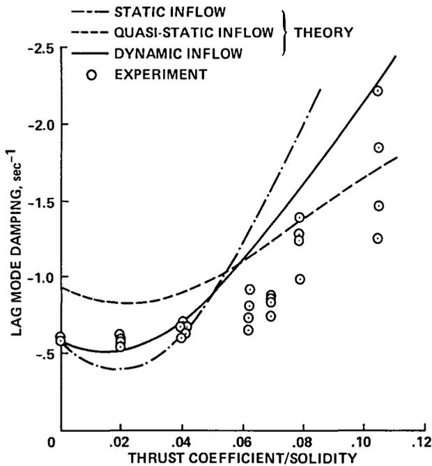
Fig. 86. Soft-inplane hingeless rotor stability with dynamic inflow (Ref. 30).
