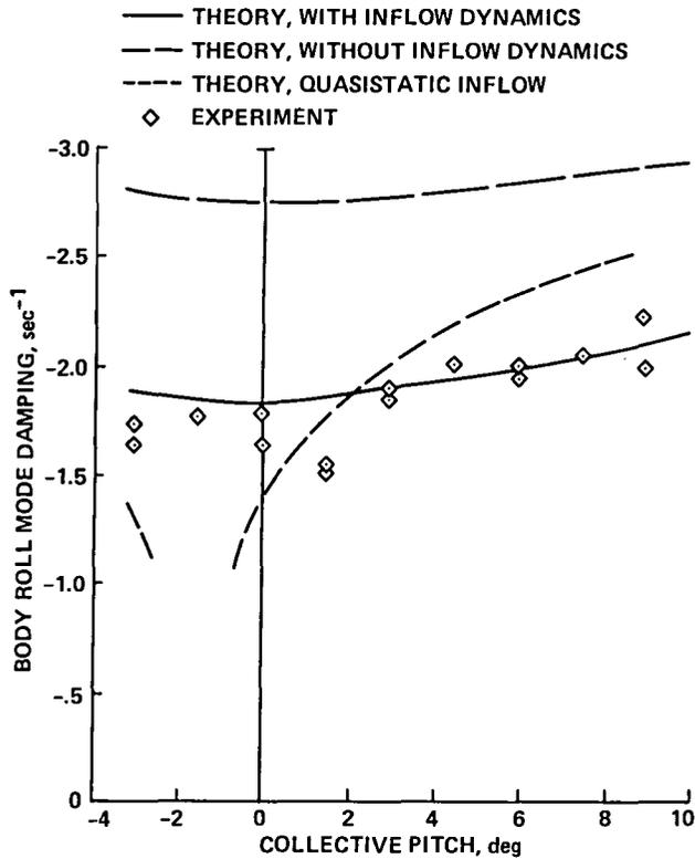
Fig. 83. Ground resonance stability with dynamic inflow (Ref. 80).
