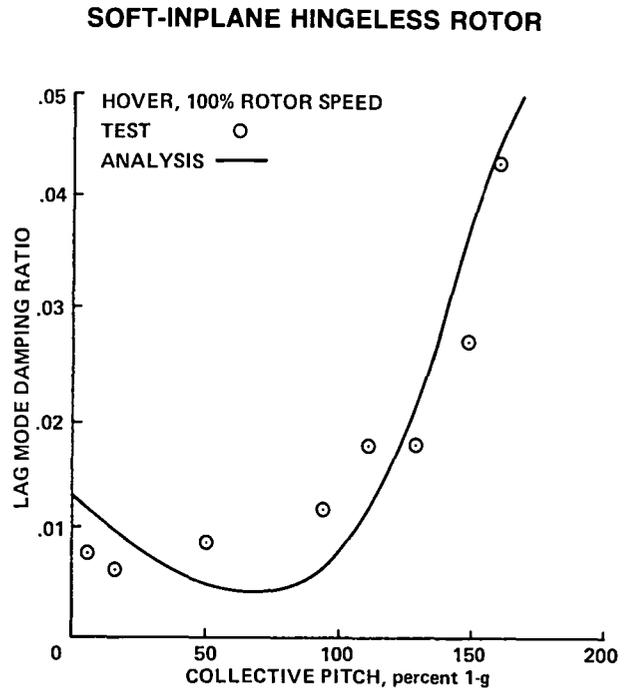
Fig. 12. Soft-inplane hingeless rotor air resonance damping (Ref. 13).
