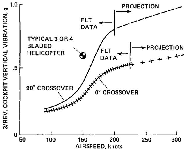
Fig. 100. Measured ABC rotorcraft vibration (Ref. 109).
