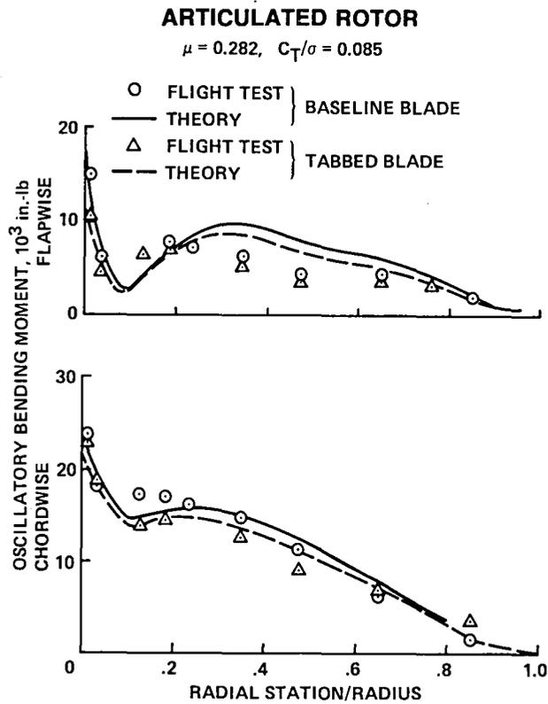
Fig. 57. Articulated rotor blade loads (Ref. 51).
