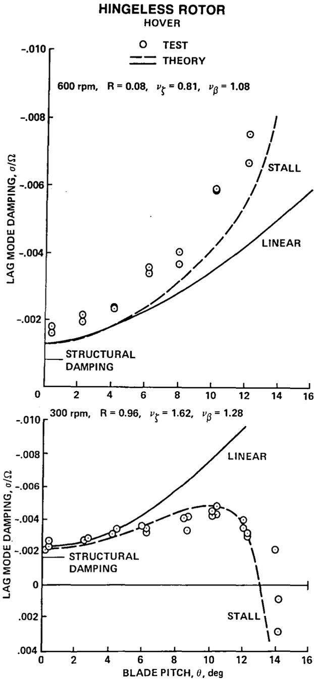
Fig. 17. Flap-lag stability produced by stall (Ref. 17).
