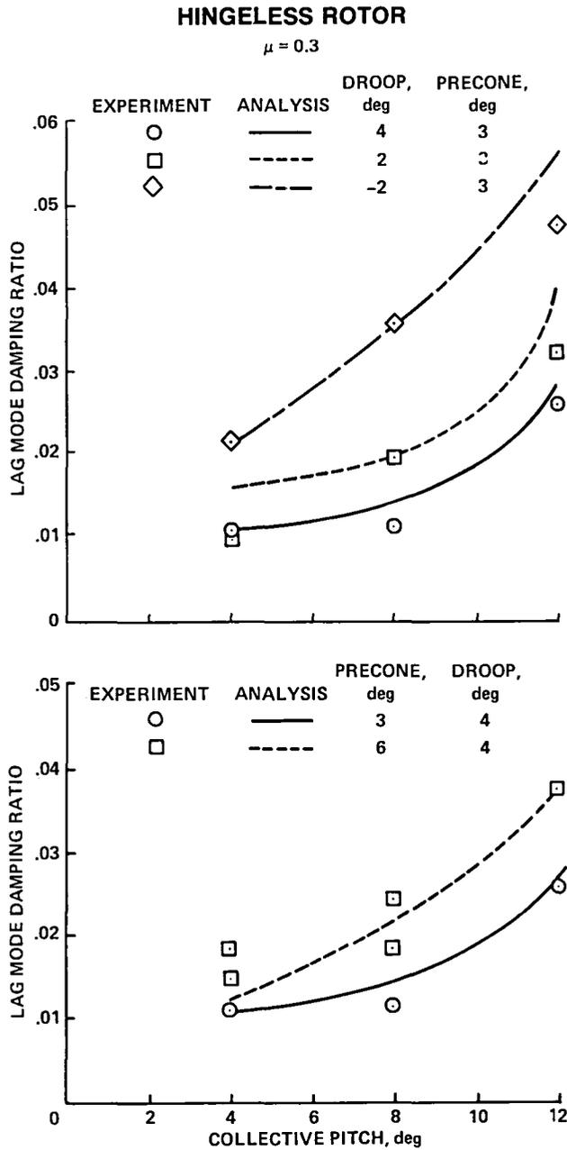
Fig. 49. Hingeless rotor ground resonance stability (Ref. 48).
