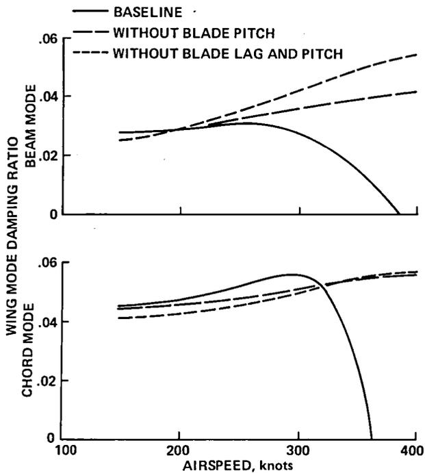
Fig. 126. Calculated tilting prop-rotor aircraft whirl flutter stability.
