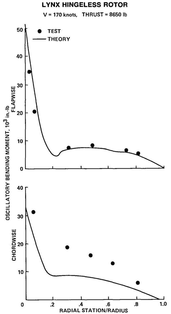
Fig. 54. Hingeless rotor blade loads (Ref. 56).
