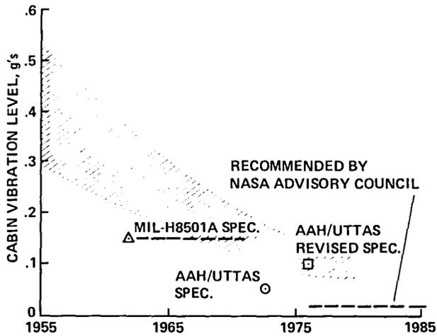
Fig. 65. Trend of helicopter vibration levels (Ref. 64).
