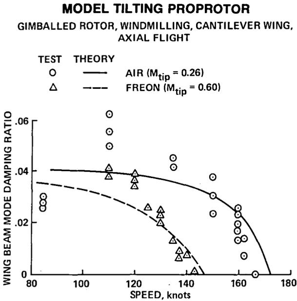
Fig. 131. Model tilting propotor whirl flutter stability (Ref. 144).
