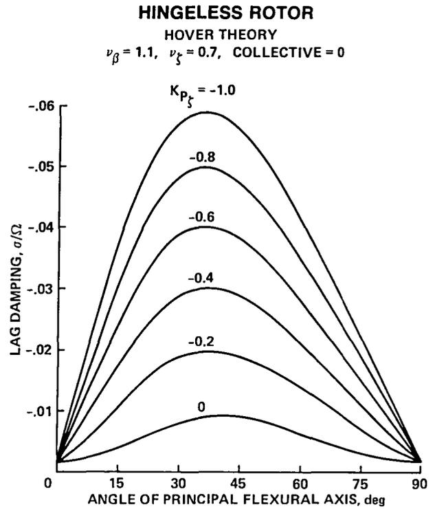
Fig. 14. Calculated hingeless rotor stability (Ref. 15).
