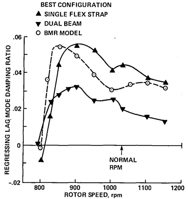
Fig. 113. Measured model bearingless rotor stability (Ref. 116).
