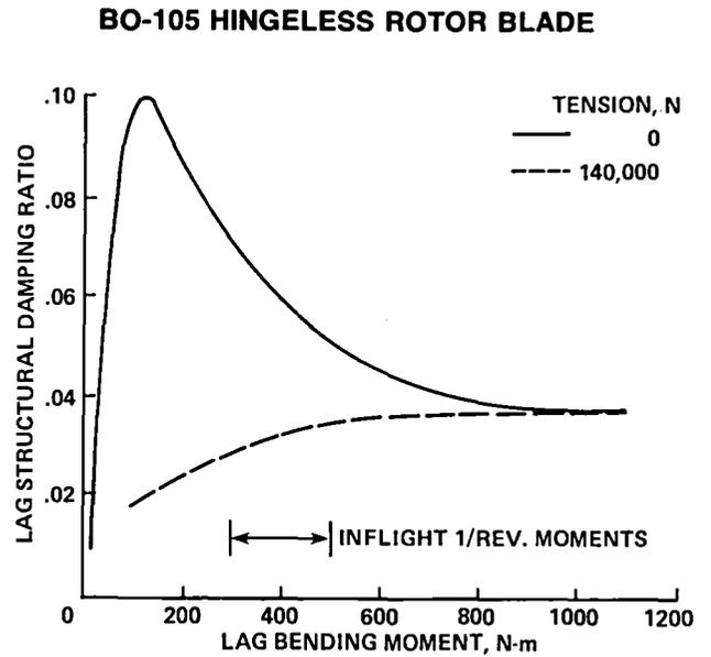
Fig. 95. Measured BO-105 blade structural lag damping (Ref. 98).
