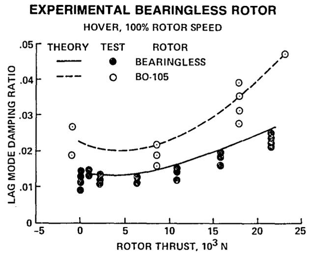
Fig. 116. Experimental bearingless rotor stability (Ref. 102).
