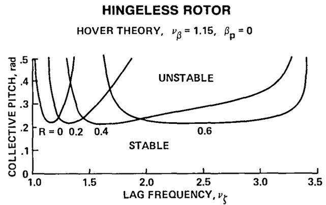
Fig. 20. Calculated elastic flap-lag stability boundaries (Ref. 24).
