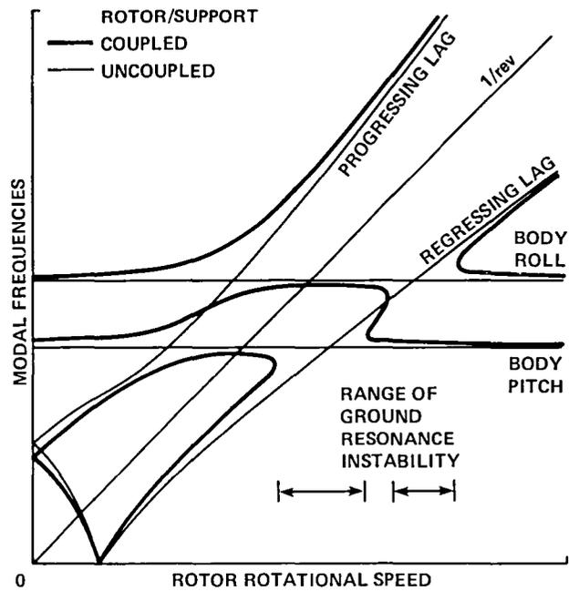
Fig. 2. Coleman diagram for ground resonance.
