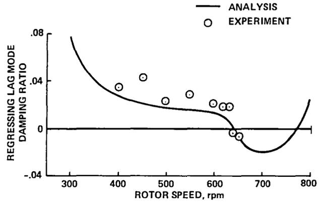
Fig. 48. Hingeless rotor ground resonance stability (Ref. 48).
