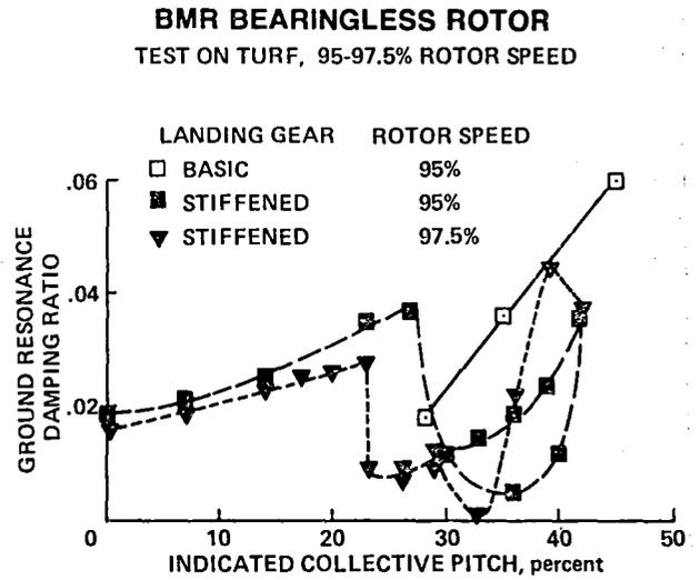
Fig. 109. Measured BMR bearingless helicopter stability (Ref. 113).
