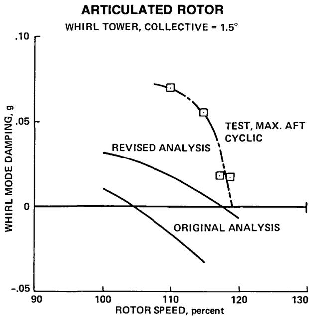
Fig. 124. Articulated rotor whirl mode stability (Ref. 137).
