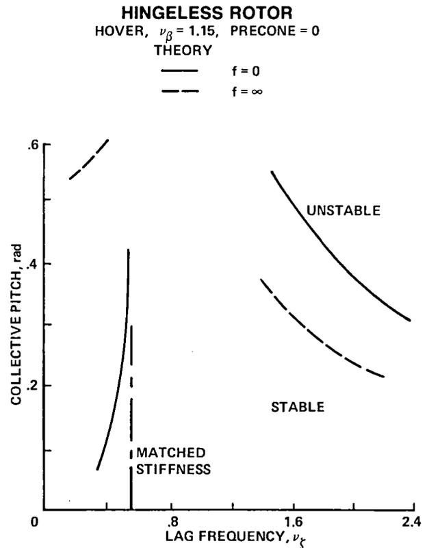
Fig. 27. Calculated pitch-flap-lag-torsion stability boundaries (Ref. 27).
