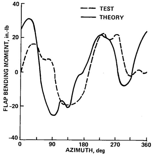
Fig. 60. Articulated rotor blade loads (Ref. 60).
