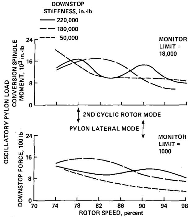
Fig. 132. Measured XV-15 Tilting Proprotor Research Aircraft pylon loads (Ref. 145).
