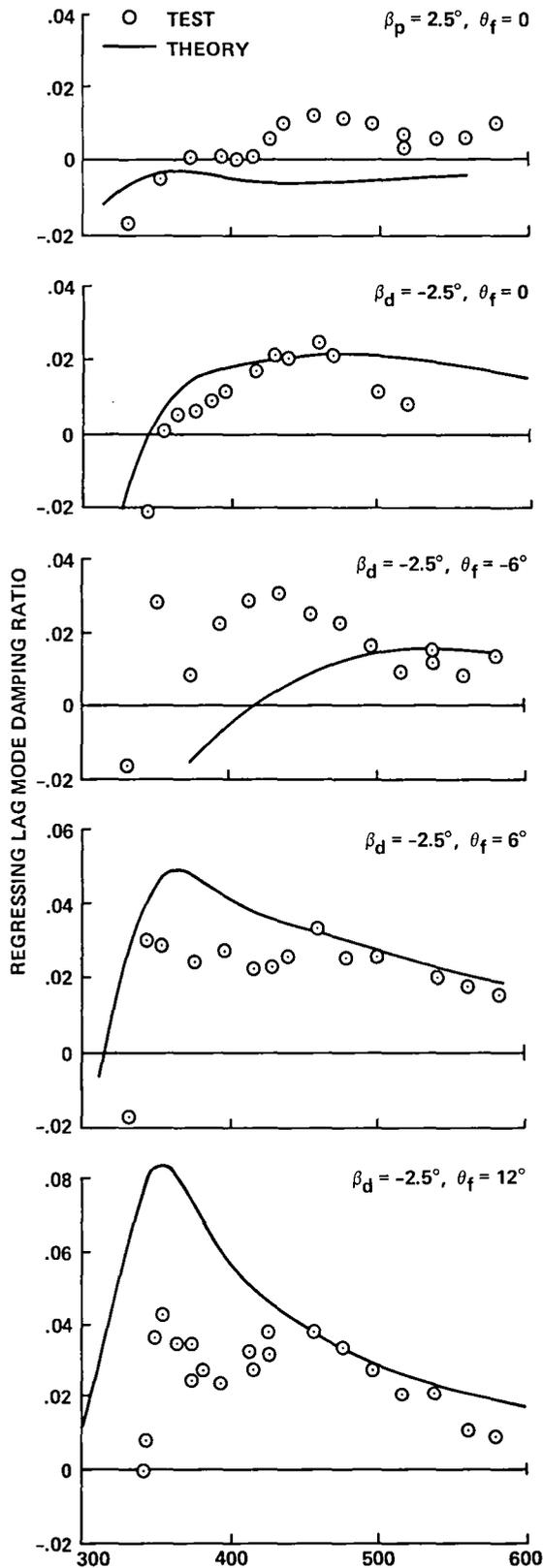
Fig. 39. Bearingless rotor stability (Ref. 39).
