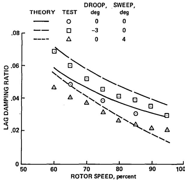
Fig. 114. Small scale Model 680 bearingless rotor stability (Ref. 119).
