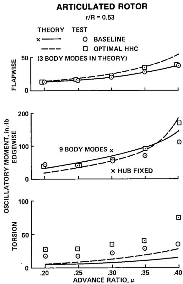
Fig. 61. Articulated rotor blade loads (Ref. 63).
