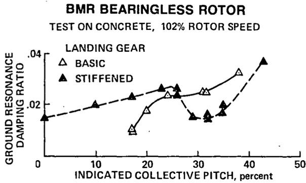
Fig. 108. Measured BMR bearingless helicopter stability (Ref. 113).
