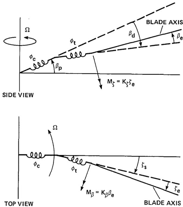
Fig. 1. Origin of effective pitch/lag and pitch/flap coupling.
