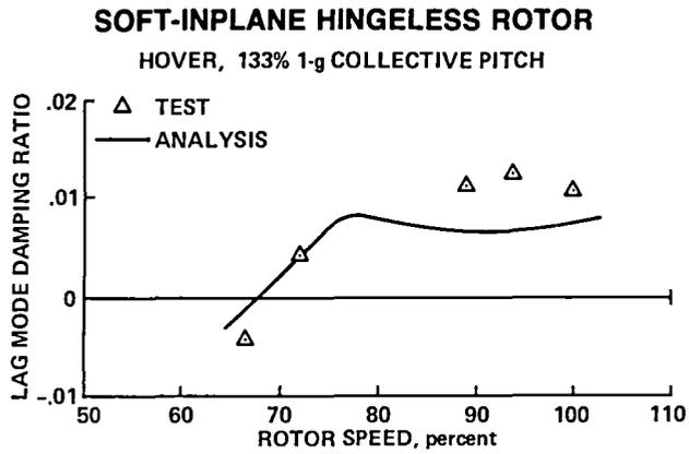
Fig. 13. Soft-inplane hingeless rotor air resonance damping (Ref. 13).
