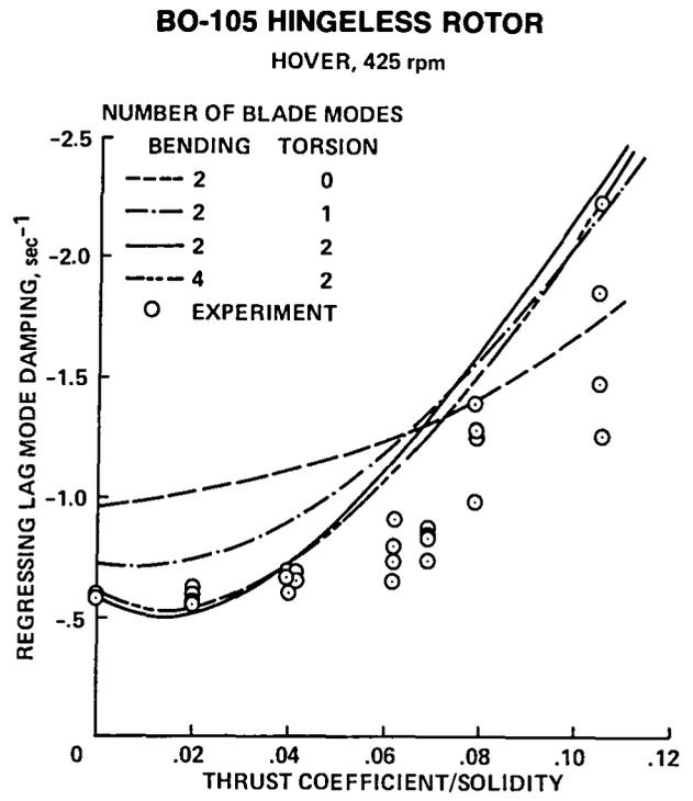
Fig. 29. Soft-inplane hingeless rotor stability (Ref. 30).
