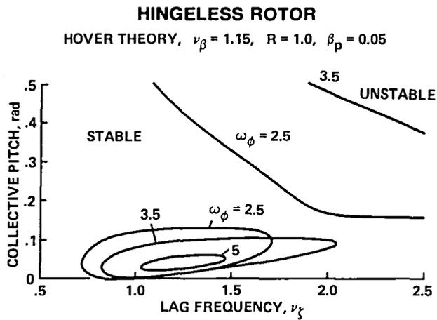
Fig. 22. Calculated flap-lag-torsion stability boundaries (Ref. 24).
