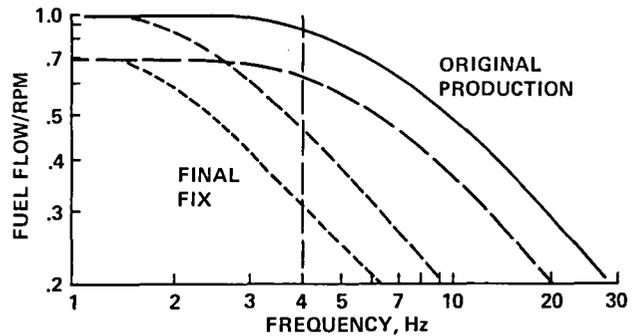
Fig. 123. Fuel control frequency response (Ref. 134).
