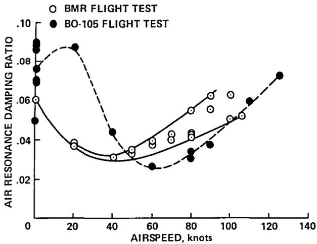
Fig. 106. Measured BMR bearingless helicopter stability (Ref. 113).
