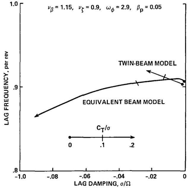
Fig. 45. Calculated bearingless rotor root locus (Ref. 44).
