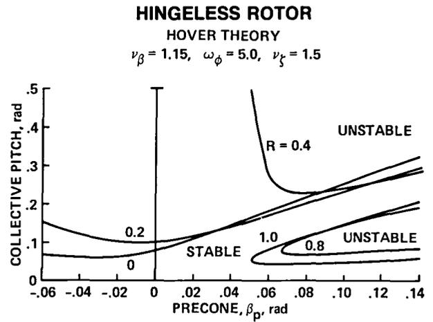
Fig. 23. Calculated flap-lag-torsion stability boundaries (Ref. 24).
