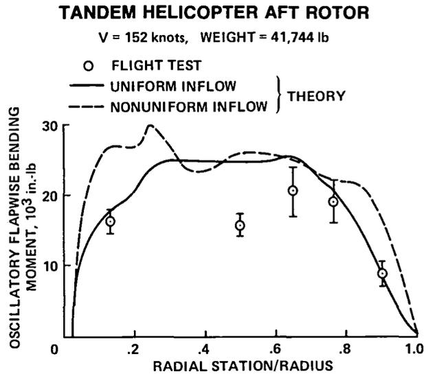
Fig. 50. Articulated rotor blade loads (Ref. 52).
