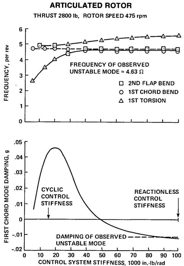
Fig. 125. Articulated rotor blade stability (Ref. 138).
