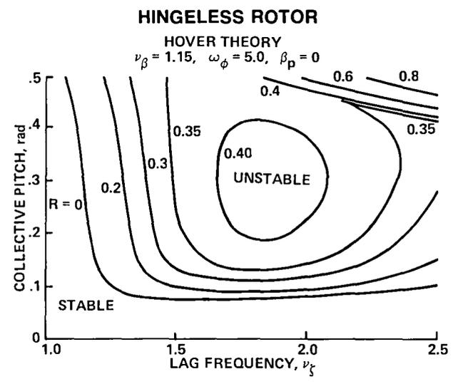
Fig. 21. Calculated flap-lag-torsion stability boundaries (Ref. 24).
