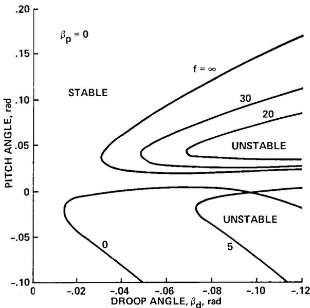
Fig. 25. Calculated pitch-flap-lag-torsion stability boundaries (Ref. 26).
