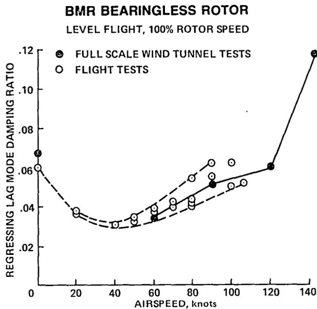
Fig. 110. Measured BMR bearingless helicopter stability (Ref. 41).
