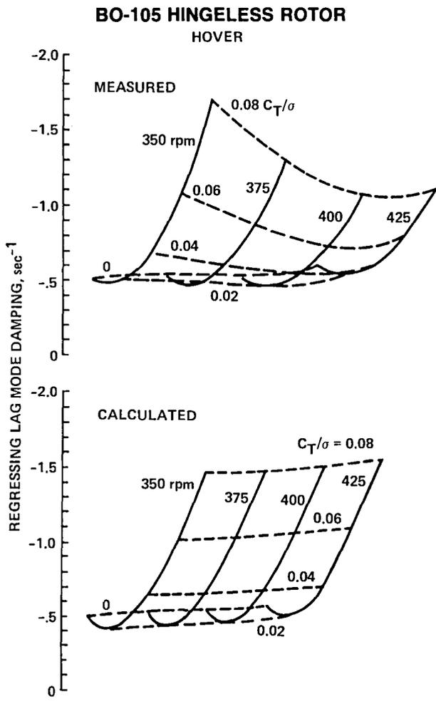
Fig. 30. Soft-inplane hingeless rotor stability (Ref. 30).
