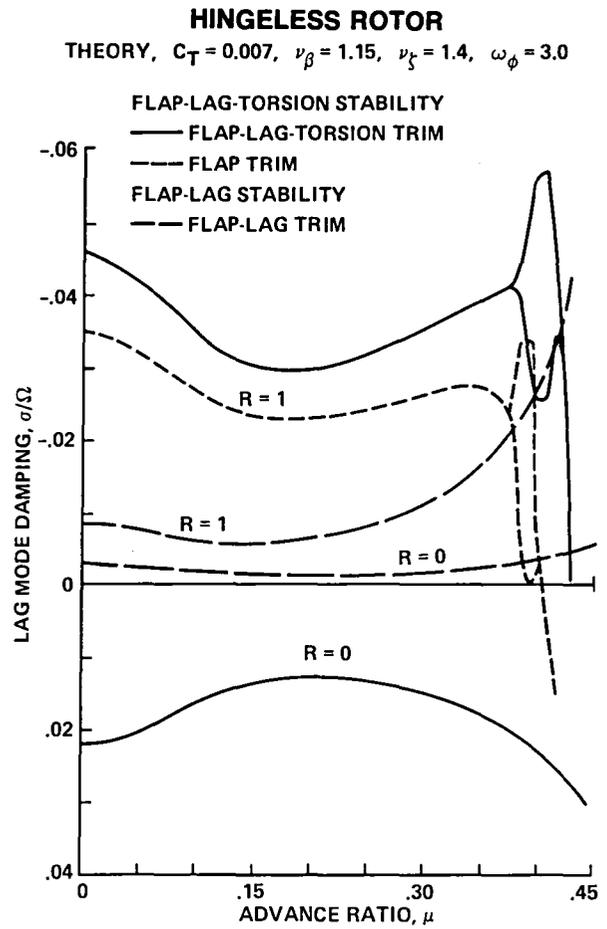
Fig. 38. Calculated elastic flap-lag-torsion stability (Ref. 35).
