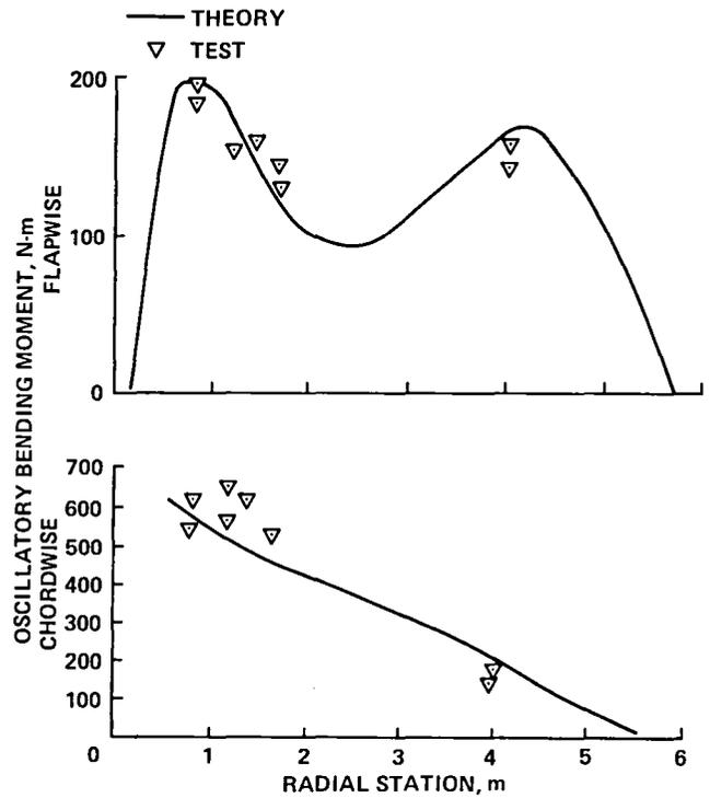
Fig. 52. Semi-rigid rotor blade loads (Ref. 54).
