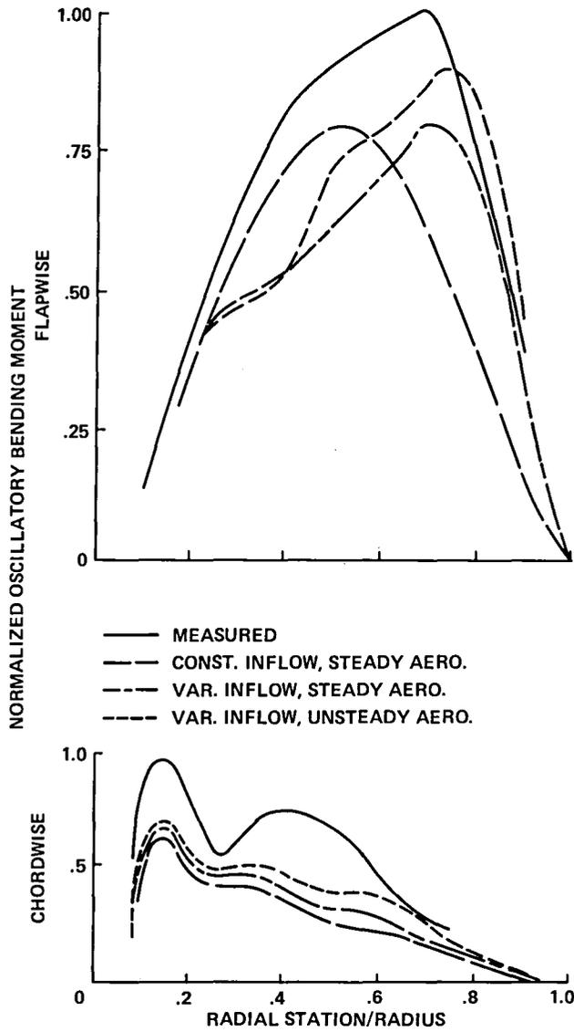
Fig. 51. Articulated rotor blade loads (Ref. 53).
