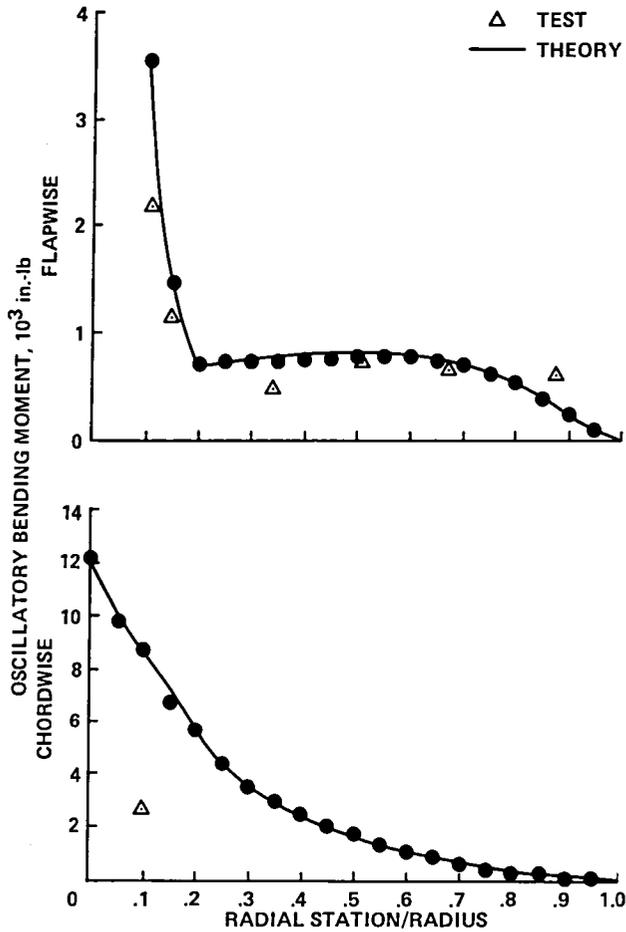
Fig. 59. Hingeless rotor blade loads (Ref. 59).
