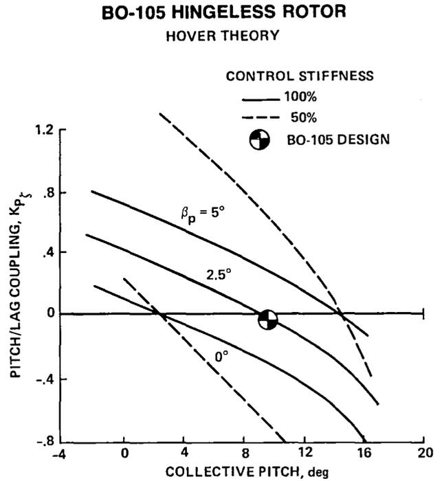
Fig. 10. Calculated pitch/lag coupling for BO-105 helicopter (Ref. 12).
