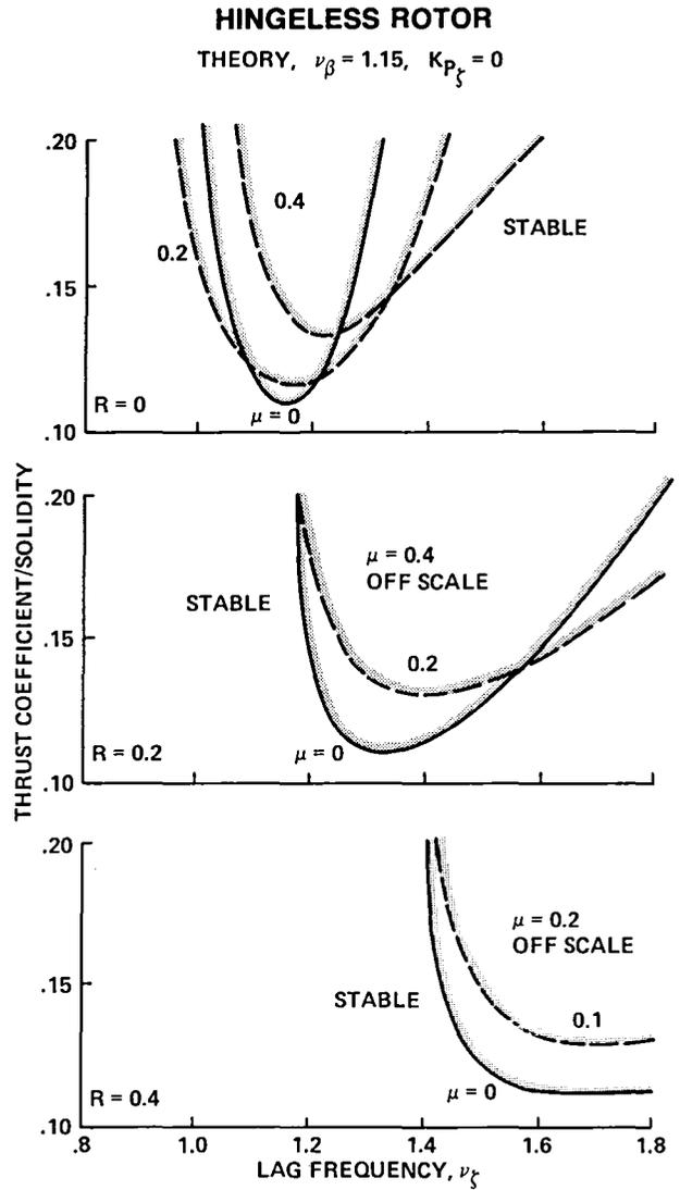
Fig. 34. Calculated flap-lag stability boundaries (Ref. 31).
