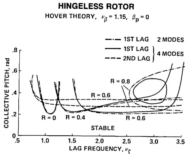
Fig. 24. Calculated elastic flap-lag stability boundaries (Ref. 25).
