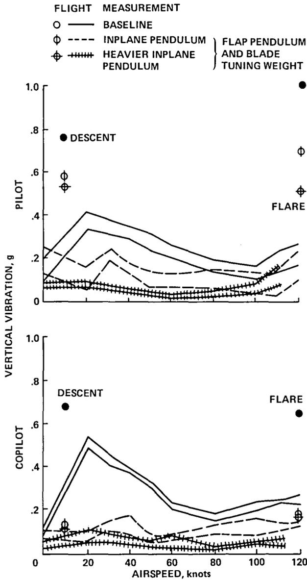
Fig. 73. Measured hingeless rotor vibration reduction (Ref. 68).
