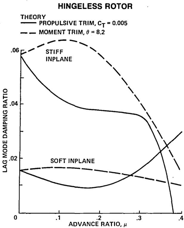
Fig. 37. Calculated elastic flap-lag-torsion stability (Ref. 34).
