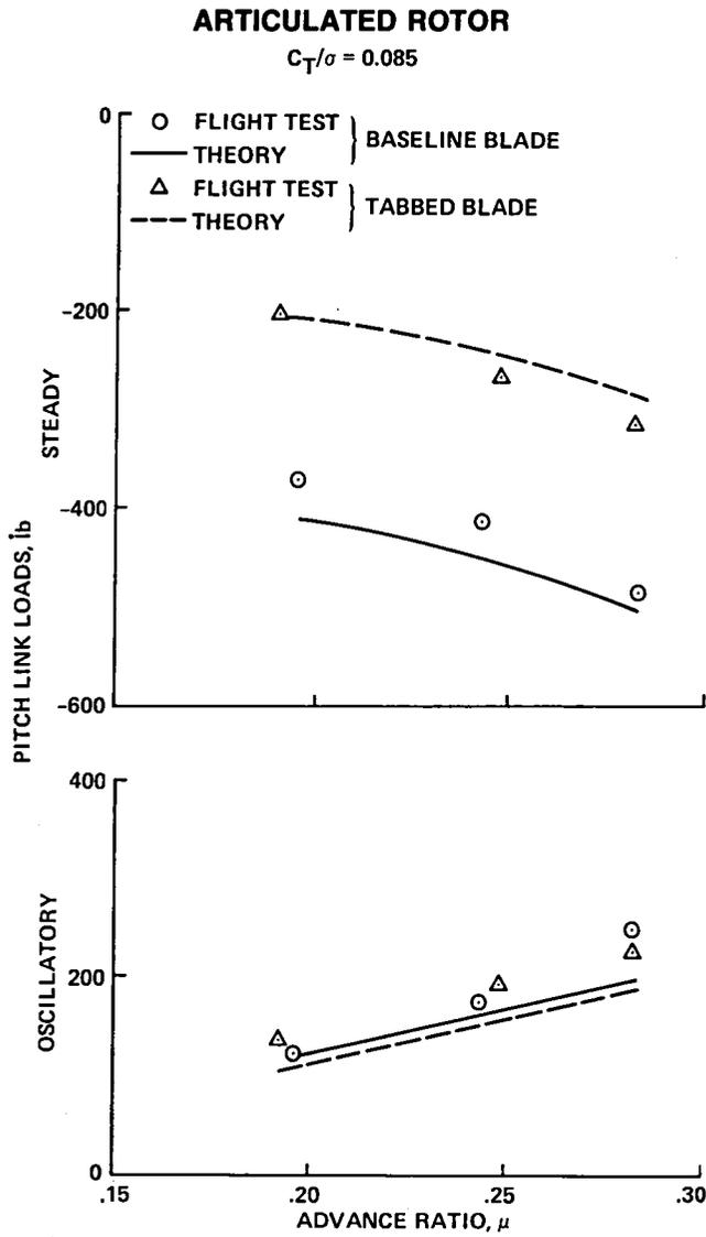
Fig. 63. Articulated rotor blade loads (Ref. 51).
