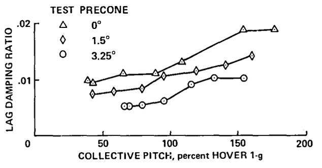
Fig. 31. Measured soft-inplane hingeless rotor air resonance stability (Ref. 13).
