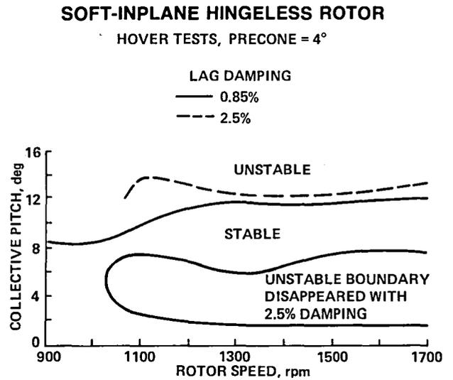
Fig. 8. Measured soft-inplane hingeless rotor stability boundaries (Ref. 10).
