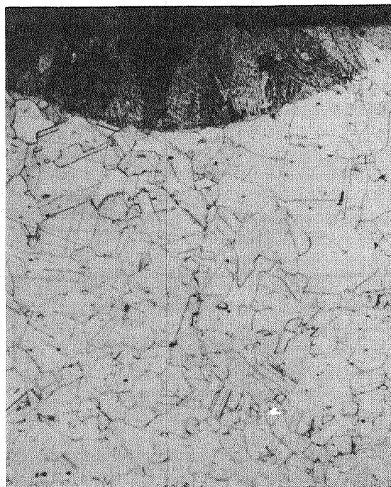
Fig. 12. Inconel 718 that has been Pre-cracked, EB Welded, HIPed, and Reheat Treated. The EB Weld is at the Top of the Photograph. A Trace of the Healed Crack is Evident in the Center.
