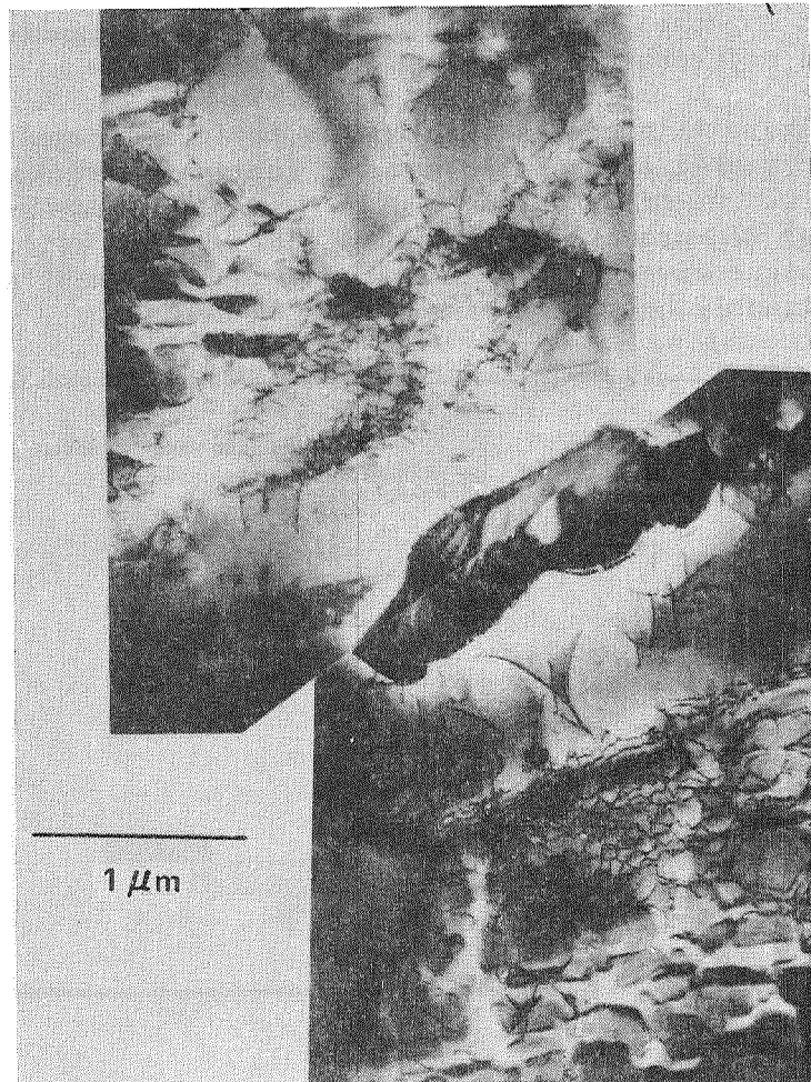
Fig. 10. TEM Micrograph of Fatigue Damage in MAR-M246(Hf) (DS) in the Vicinity of a Tungsten Carbide. Fatigue Exposure: 359 MPa (52 ksi), R = -1, 843 C (1550 F), 442,000 Cycles (70 Percent of Mean Life)
