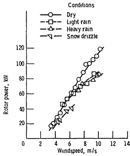
Figure 6 - Rotor performance for configuration II
