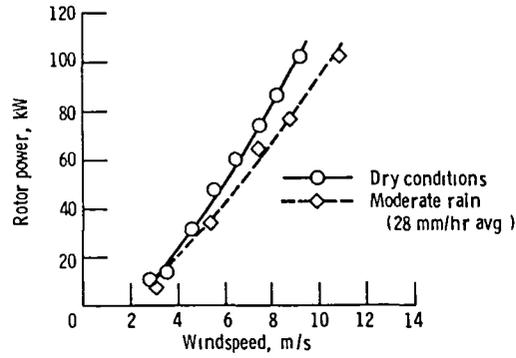
Figure 7 - Rotor performance for configuration III
