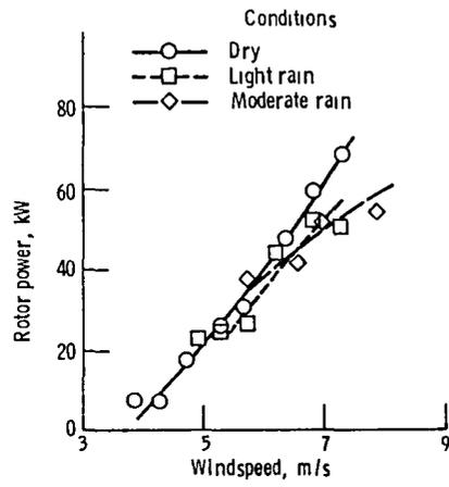
Figure 5 - Rotor performance for configuration I
