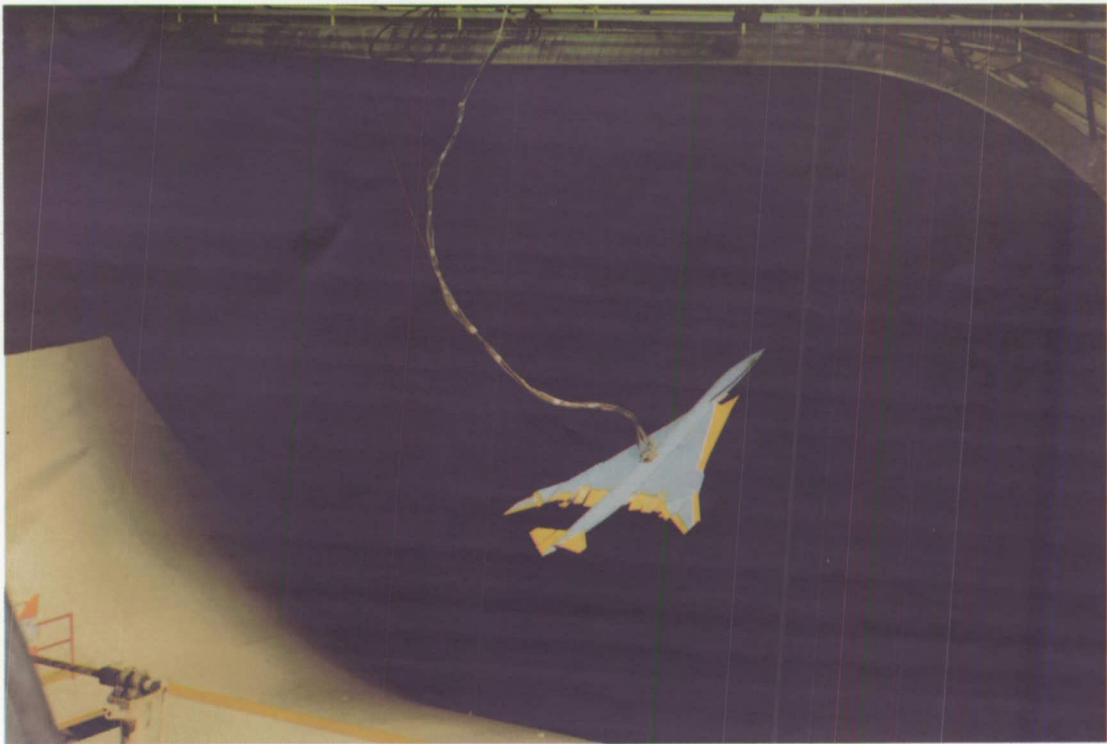
Tethered free-flight tests of SCR arrow-wing model in Langley Research Center full-scale wind tunnel. Findings: (a) model longitudinally stable over test \alpha range; (b) coupled roll and yaw control provided effective lateral control up to \alpha = 27^\circ .
