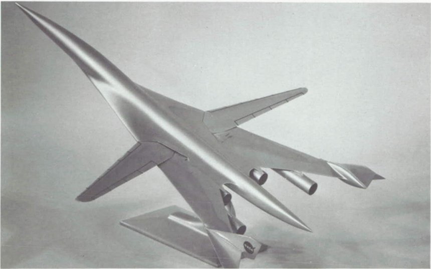
NASA SST feasibility concept — the variable-sweep SCAT-15 with blended body and interlocking wings (forerunner of the fixed-wing SCAT-15F.)
