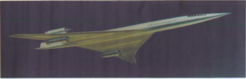
Lockheed reference airplane for SCR technology assessment. Note over/under engine locations on wing.
