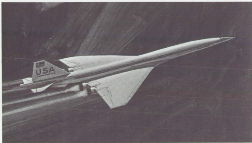
Boeing B2707-300 with four GE-4 engines — the proposed U.S. SST at the time program was canceled.
