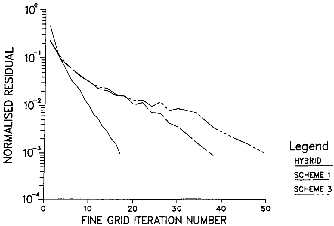
Fig. 18. Rates of Convergence, Re = 600 , 20x20 Grid
