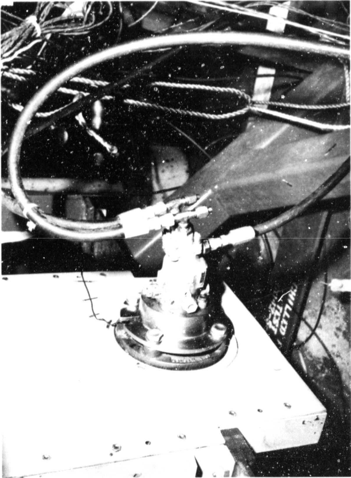
Figure 7. Vibrator Hydraulic Drive Motor
