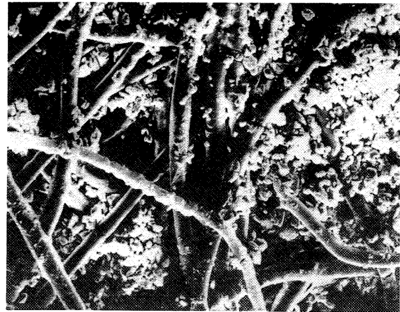
SEM OF NEG # 3 WITH SEPARATOR 320 X
