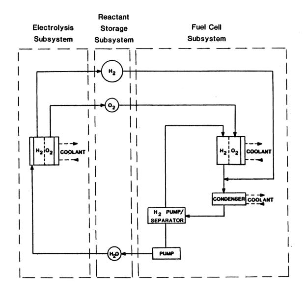
Figure 5. RFC system schematic diagram
