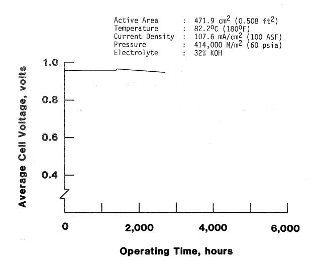
Figure 2. UTC four-cell stack endurance test
