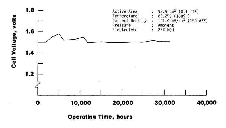
Figure 3. LSI single cell endurance test
