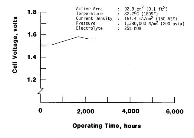
Figure 4. LSI six-cell stack endurance test
