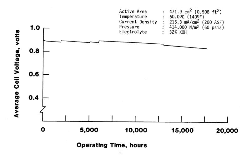
Figure 1. UTC six-cell stack endurance test
