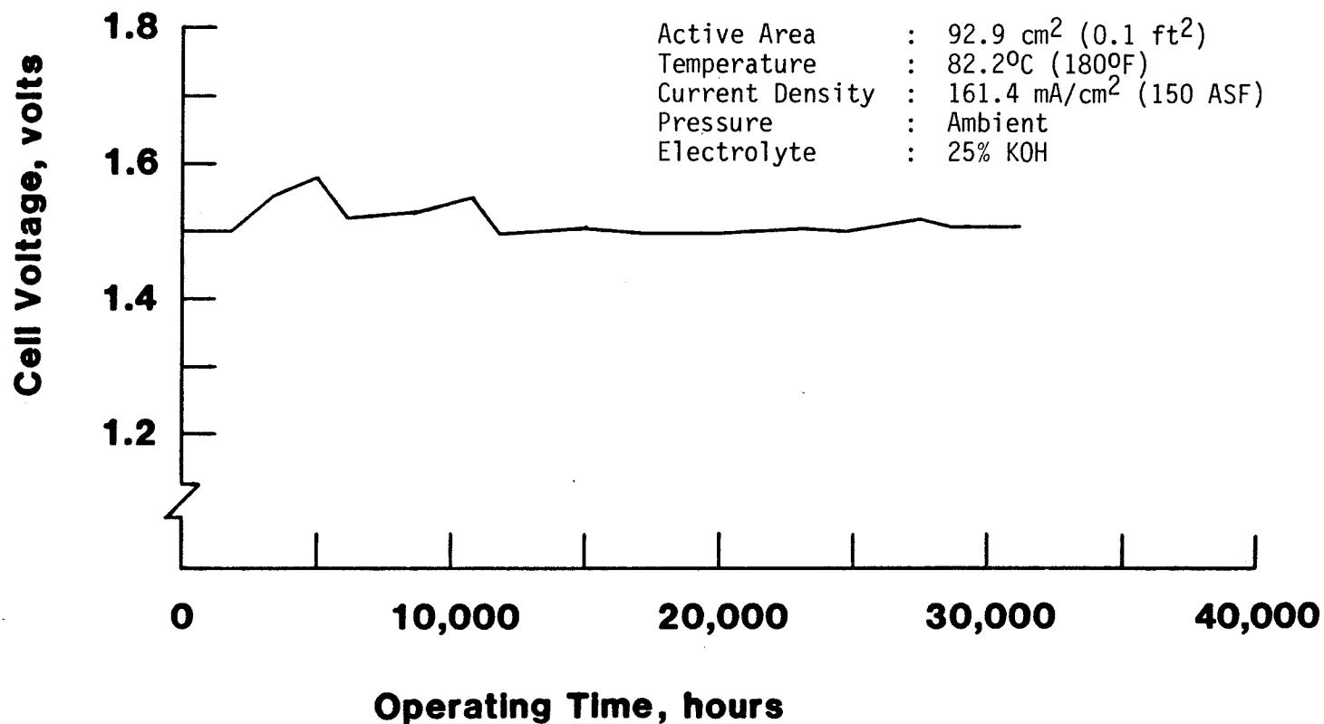
Figure 3. LSI single cell endurance test
