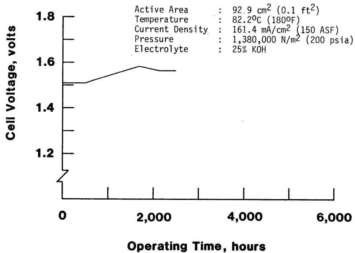
Figure 4. LSI six-cell stack endurance test
