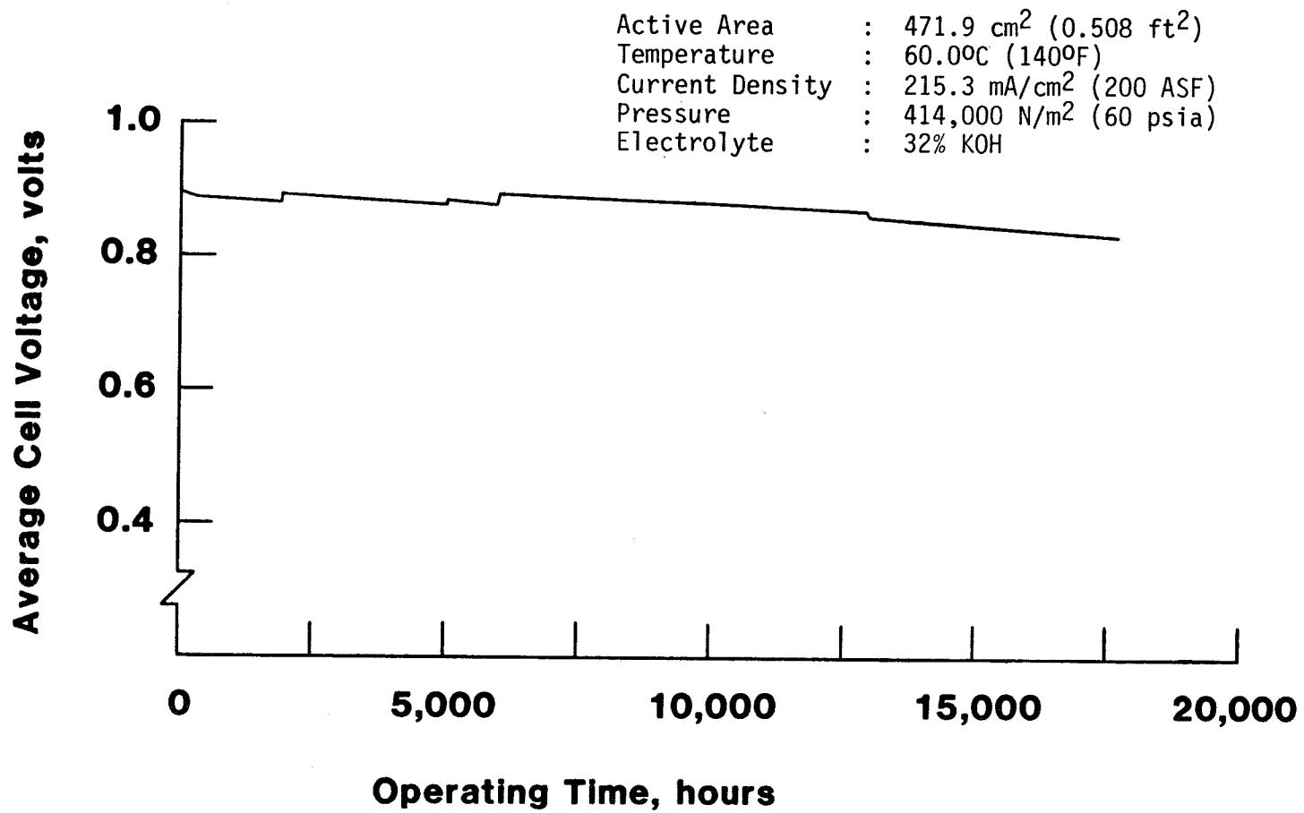
Figure 1. UTC six-cell stack endurance test
