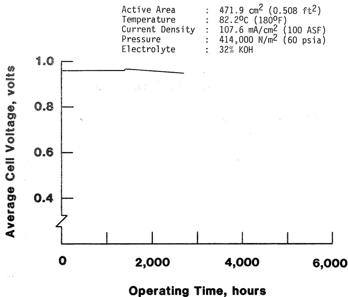
Figure 2. UTC four-cell stack endurance test
