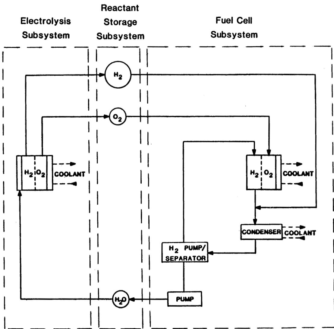
Figure 5. RFC system schematic diagram
