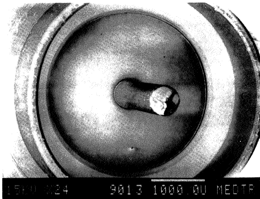
Figure 4. Glass Seal From Fresh Battery.
