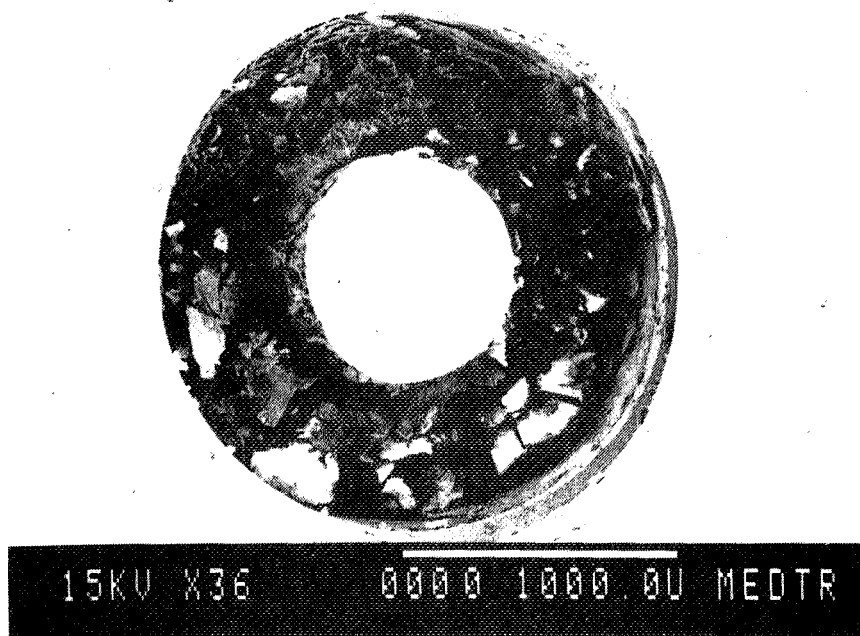
Figure 5. Glass Seal After Exposure to Liquid Electrolyte
