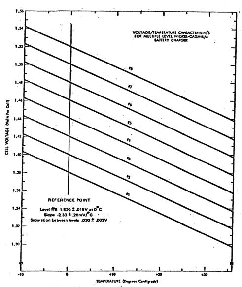
Cell Voltage Limit versus Temperature
