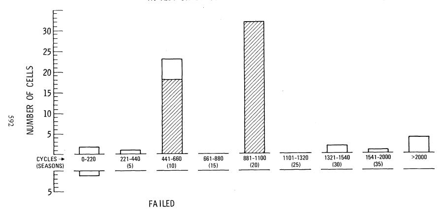
Figure 3. Distribution of testing and failures for USAF design cells in high earth orbit simulations are shown for 66 cells. The cross-hatched bars are numbers of cells in elliptical orbit simulations.
