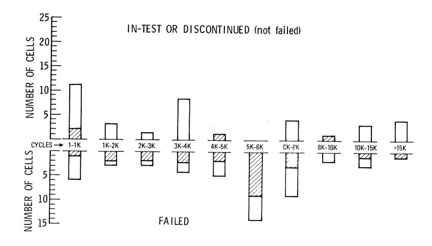
Figure 2. Distribution of testing and failures for USAF design cells in LEO simulations excluding those 42 cells in the two Air Force Flight Experiment test batteries. Cross-hatched bars are numbers of cells tested at 80% depth of discharge.
