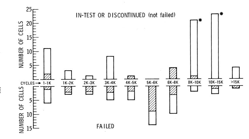
Figure 1. Distribution of testing and failures for all USAF design cells (128 cells) in low earth orbit (LEO) simulations is shown. Cross-hatched bars are numbers of cells tested at 80% depth of discharge. Asterisks indicate the major contribution from cells in the two USAF Flight experiment batteries.
