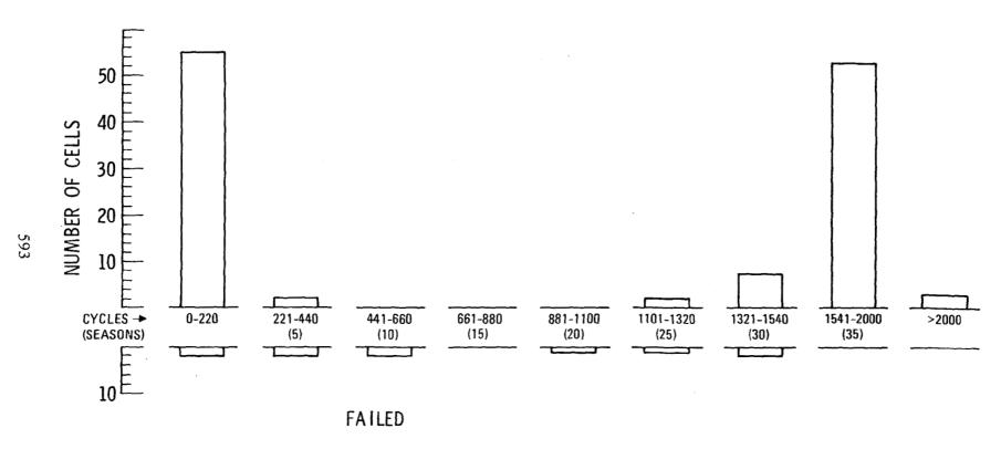
Figure 4. Distribution of testing and failures for COMSAT design cells in geostationary orbit simulations are shown for 132 cells.
