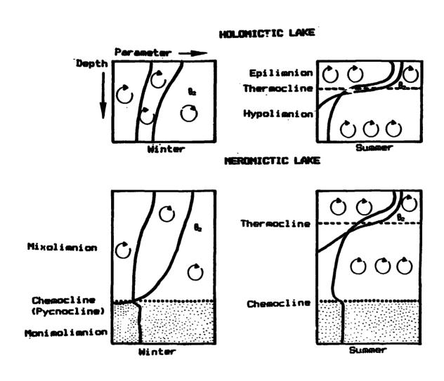
Figure I-13. Vertical structure of the water column in lakes of temperate regions. When sulfide and light are present massive populations of phototrophic sulfur bacteria can develop at the hypolimnion during the summer and in the monimolimnion of meromictic lakes during the remainder of the year.
