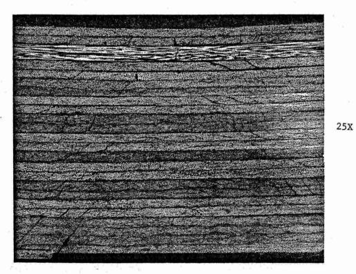
Figure 4-48: Sectional Micrographs of Specimen 14-2 Impacted At 15 Ft.-Lbs.
