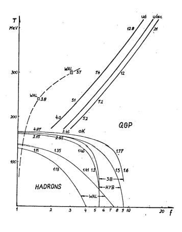
Temperature T and compression factor (f) of nuclear fireball together with phase diagram for Walecka (WAL), Hybrid (HYB) and stat. Bootstrap (SB) models of hadronic gas. T-f curve for hadronic fireball has been got for ud, uds and udsc flavours. WALcurve has been got when compressed matter is assumed to be Walecka nuclear matter. K is "Kajantie point". All numbers refer
