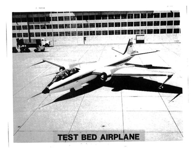
A B-57B was utilized as the sampling test bed. The aircraft was selected because of its rugged design, broad flight envelope, ease of flying and availability. The wing tip probes located 60 ft. apart are mounted at locations designed to accept fuel pods.
