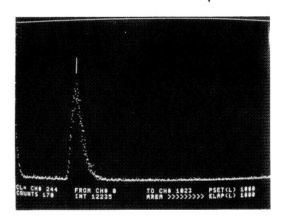
Figure 3: Velocity histogram obtained using new anemometer on air flow in a small wind tunnel. The pulse separation is converted to a pulse height and then stored on a pulse height analyzer.
