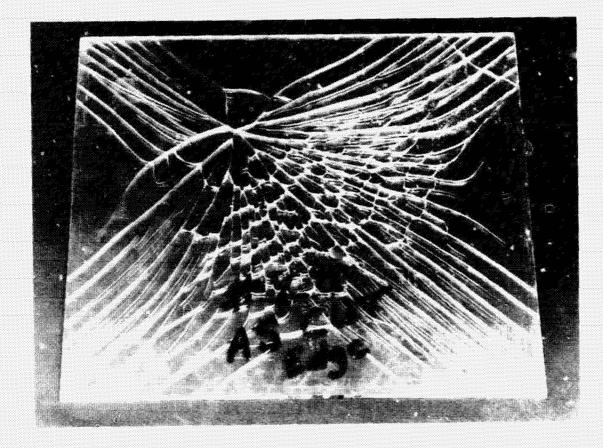
0.042 x 11.8 x 11.8-in. Annealed Glass Plate With Rounded Edges and TiO Conductive Coating; Failed at 0.90 lb/in.<sup>2</sup>
