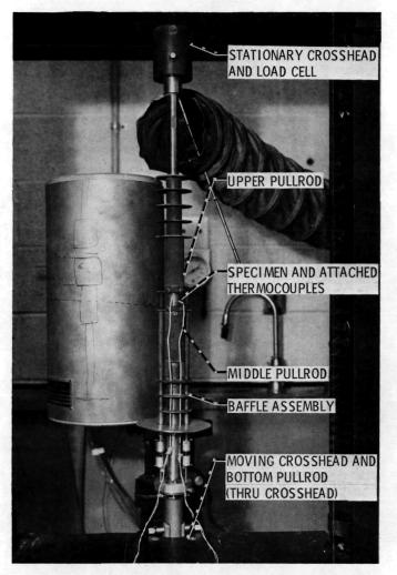
Figure 2. - Assembled text fixture mounted in load frame.
