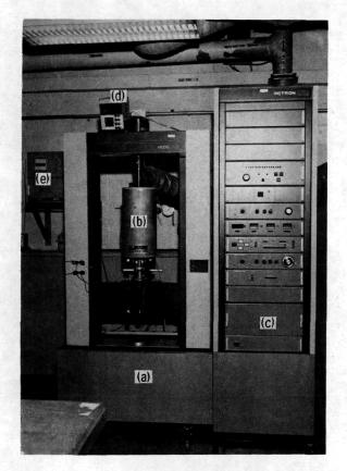
Figure 1. - Experimental setup: (a) Load frame, (b) furnace, (c) load control system and chart recorder, (d) temperature indicator and, (e) temperature controller.
