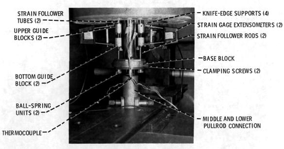
Figure 4. - Fitting of strain follower elements and strain gage extensometer.
