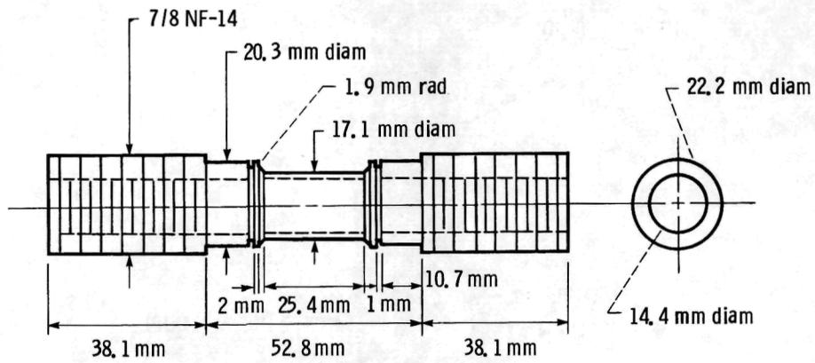
Figure 5. - Hollow tubular specimen configuration.
