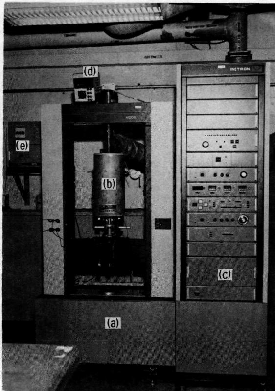
Figure 1. - Experimental setup: (a) Load frame, (b) furnace, (c) load control system and chart recorder, (d) temperature indicator and, (e) temperature controller.
