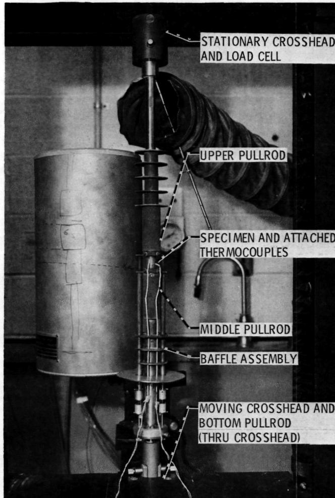
Figure 2. - Assembled test fixture mounted in load frame.
