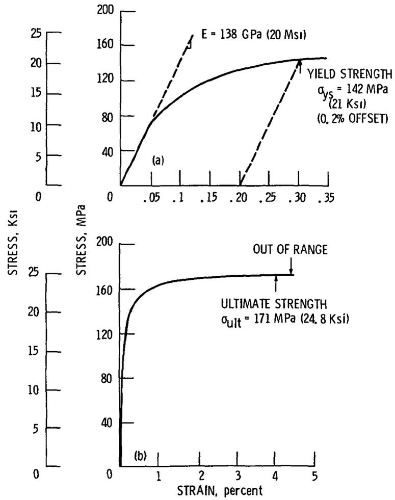
Figure 7. - Stress-strain curves of type 304 Stainless Steel tensile specimen tested at  $760^\circ\text{C (1400}^\circ\text{F)}$ .
