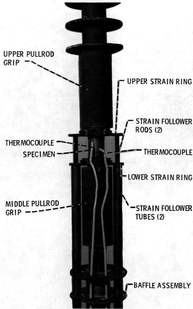
Figure 3. - Pullrods and averaging extensometry assembly with a specimen.
