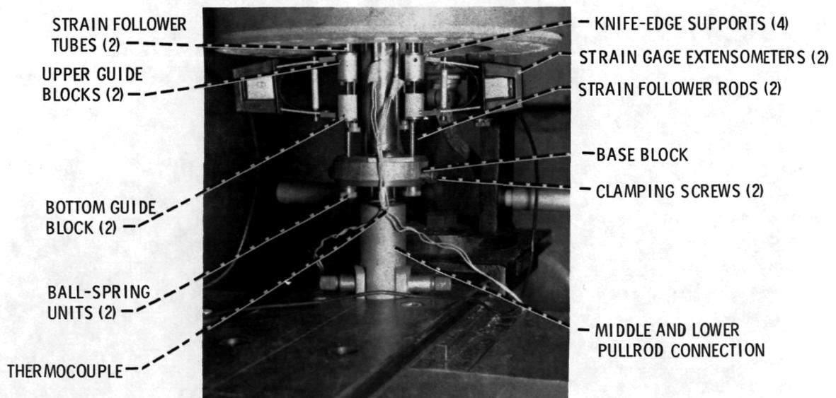
Figure 4. - Fitting of strain follower elements and strain gage extensometer.
