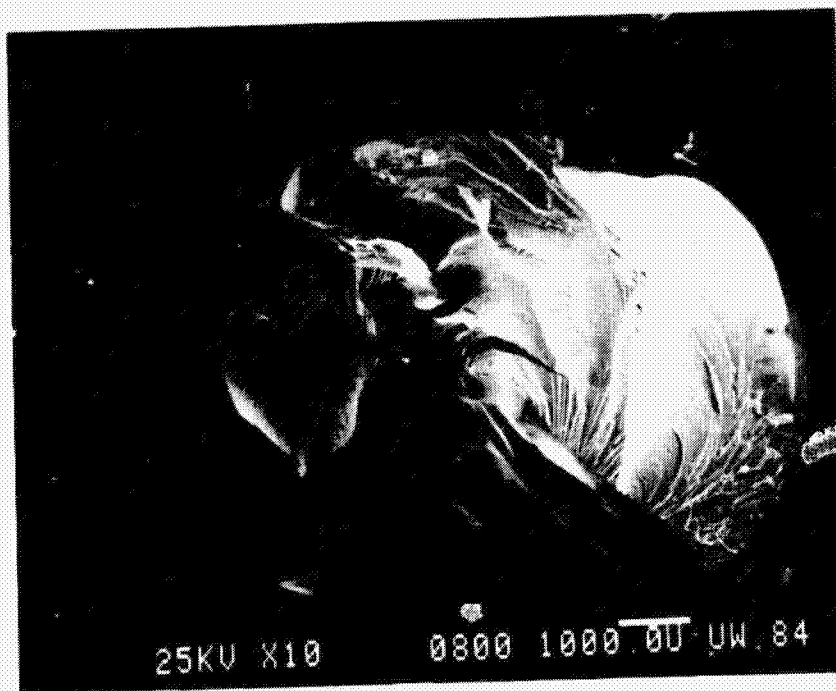
Figure D27. ERX-4901A(MDA) Epoxy Torsion Specimen No. LSDQ15, 82°C, Dry.
