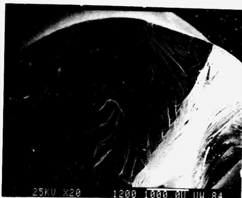
Figure D23. Narmco 5245-C Bismaleimide/Epoxy Torsion Specimen No. LSW011, 82°C, Moisture-Saturated.
