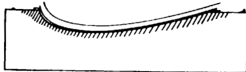
EXTERIOR FIBERGLASS SKIN WET-OUT IN BASIC MOLD
