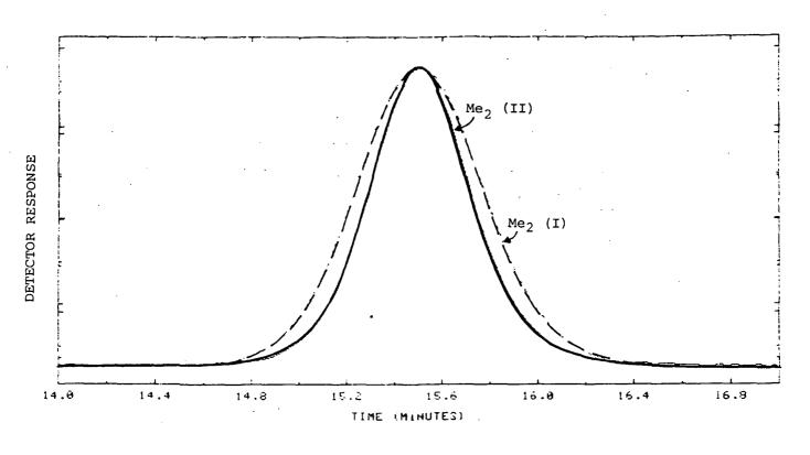
FIGURE 27. GPC Analysis - Me<sub>2</sub> (I) Before Mass Loss Measurements - Me<sub>2</sub> (II) After Mass Loss Measurements
