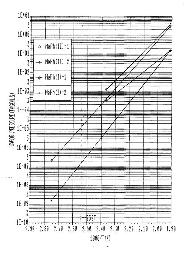
FIGURE 30. Vapor Pressure of MePh (II) and MePh (I)
