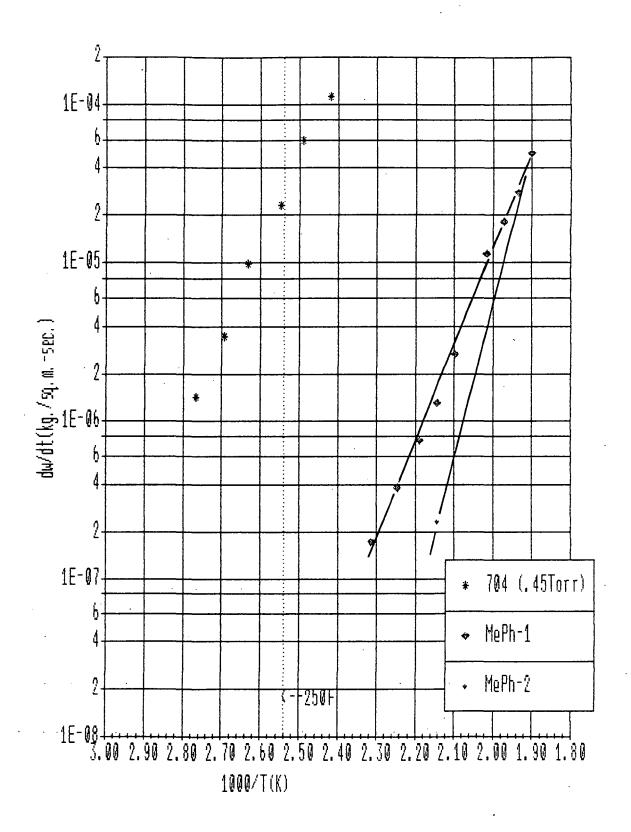
FIGURE 10d. Mass Loss Rates for MePh - (I)
