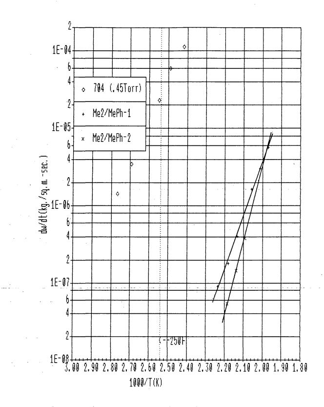
FIGURE 10a. Mass Loss Rates for  $Me_2/MePh$  - (I)
