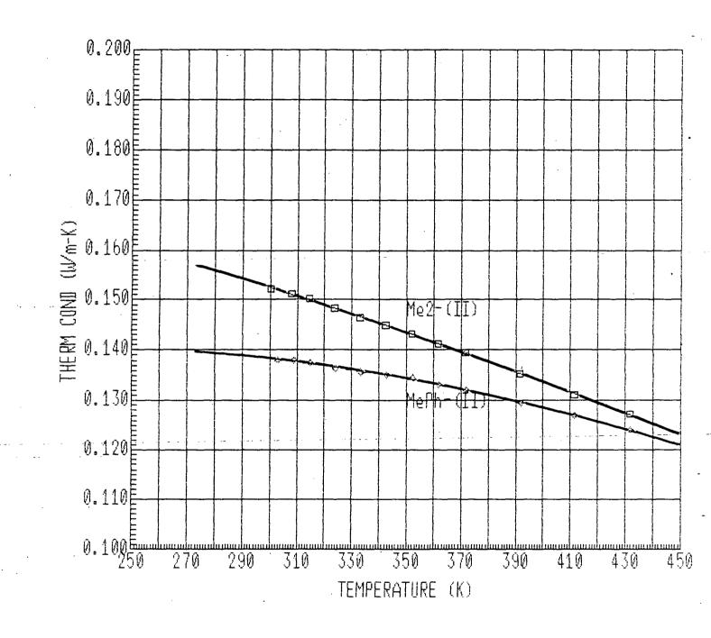
FIGURE 22. Thermal Conductivity of Task II Fluids
