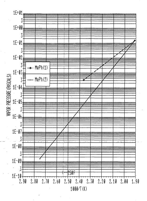
FIGURE 11d. Vapor Pressure of MePh (1), MePh (2)
