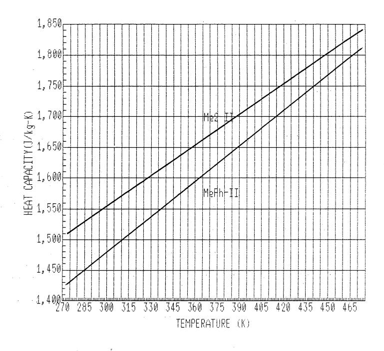
FIGURE 21. Heat Capacity of Task II Fluids
