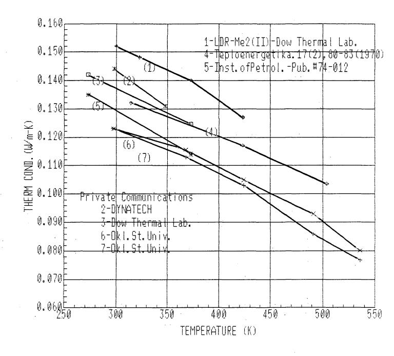
FIGURE 23. Thermal Conductivity of PDMS Fluids
