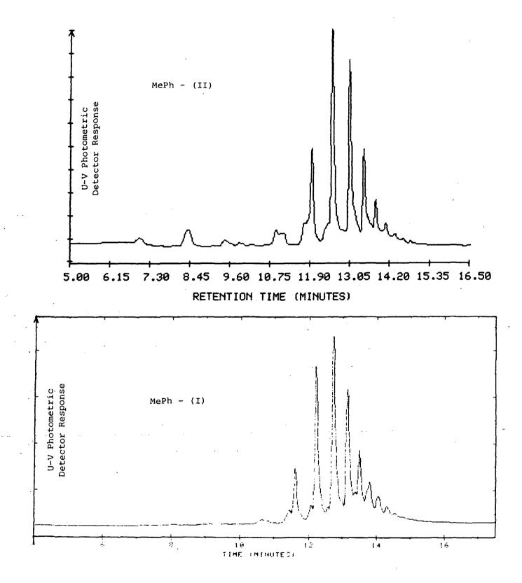
FIGURE 18. Reverse-Phase Liquid Chromatograms of MePh (I and II) Fluid
