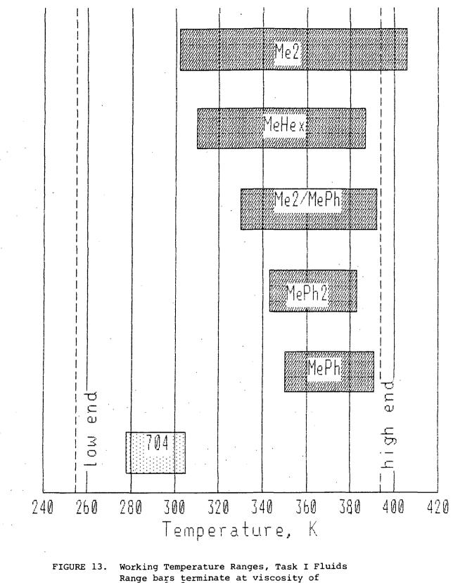
Working Temperature Ranges, Task I Fluids Range bars terminate at viscosity of 25 x  $10^{-6}$  m<sup>2</sup>/sec (low temperature) and  $10^{-7}$  Pa (high temperature) No working range exists for 704
