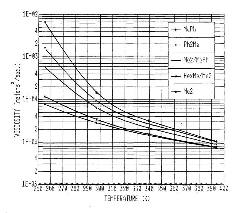
FIGURE 5. Kinematic Viscosity of Task I Fluids
