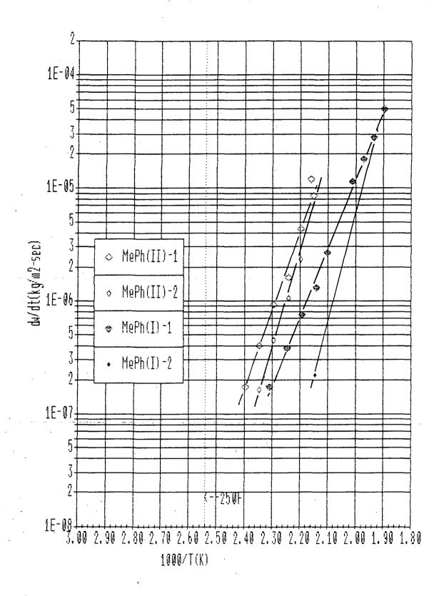
FIGURE 28. Mass Loss Rates for MePh (II) and MePh (I)
