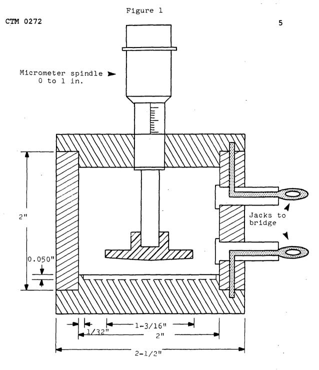
2 in. ID, 2-1/2 in. OD Teflon® tube with an opening about 1-1/2 in. wide and 3/4 in. high on the bottom edge to allow observation of the electrode and sample.
