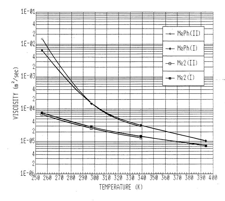
FIGURE 25. Kinematic Viscosity of Task (I and II) Fluids
