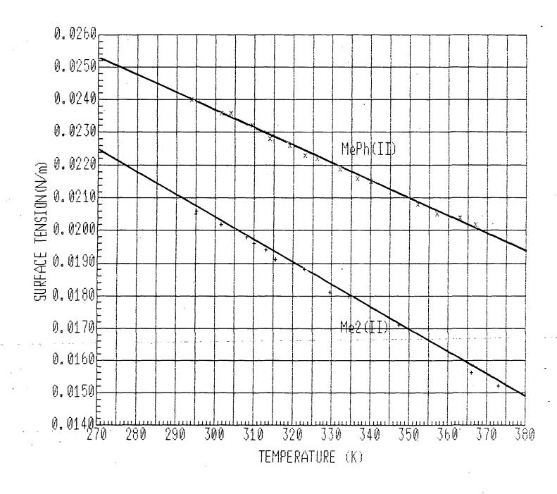
FIGURE 20. Surface Tension of Task II Fluids
