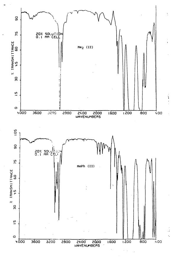
FIGURE 33a. Transmission Spectra of Task II Fluids in a 20% Solution in a 0.1mm Cell
