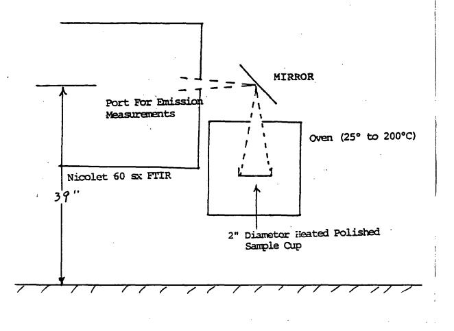
Fig. 12. Schematic drawing of oven and optical arrangement for collecting emission spectra.
