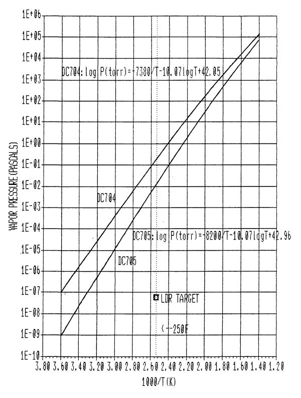
Figure 1. Vapor Pressure of DC 704, DC 705.
