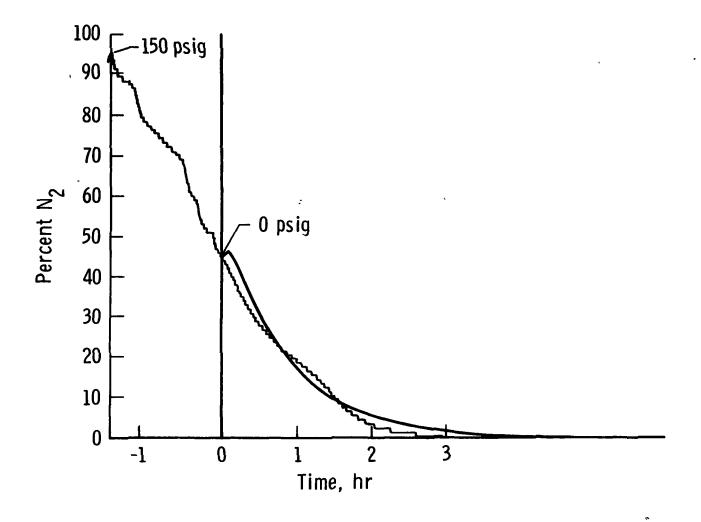
Figure 2(b). Percent  $N_2$  in Evaporated Vapor Passing Through the  $N_2$  Analyzer Versus Time: Test # 2. Wavy Line: Measured. Solid Line: Best Fit to Equation 9.
