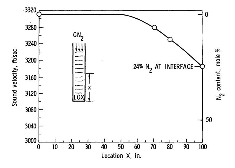
Figure 3. Contamination Profile Resulting From  $N_2$  Pressurization of LOX at 1500 psi for 5 Min, in the 7-Inch Run Tank.
