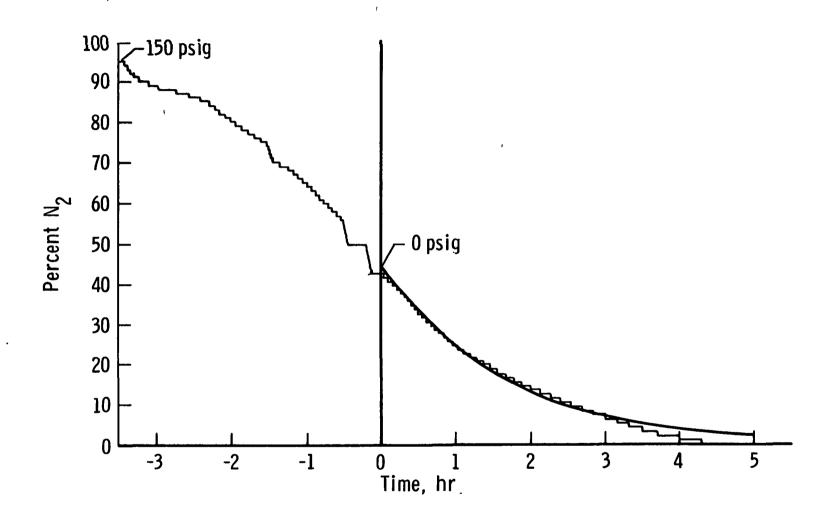
Figure 2(c). Percent  $N_2$  in Evaporated Vapor Passing Through the  $N_2$  Analyzer Versus Time: Test # 3. Wavy Line: Measured. Solid Line: Best Fit to Equation 9.
