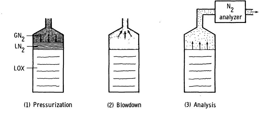
Figure 1. Illustration of the Test Procedure.
