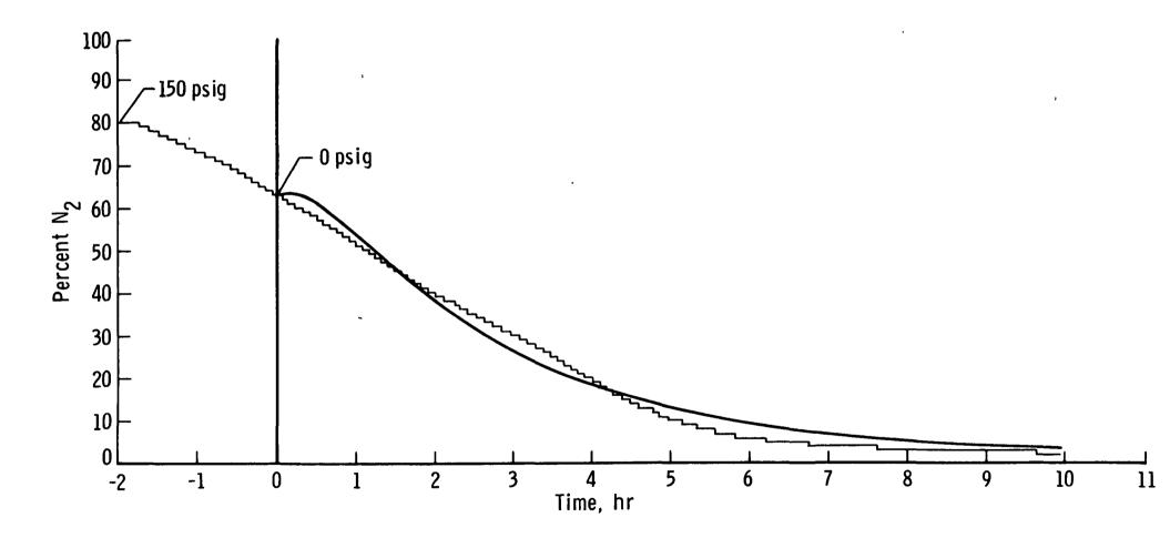
Figure 2(a). Percent  $N_2$  in Evaporated Vapor Passing Through the  $N_2$  Analyzer Versus Time: Test  $\#\ 1$ . Wavy Line: Measured. Solid Line: Best Fit to Equation 9.
