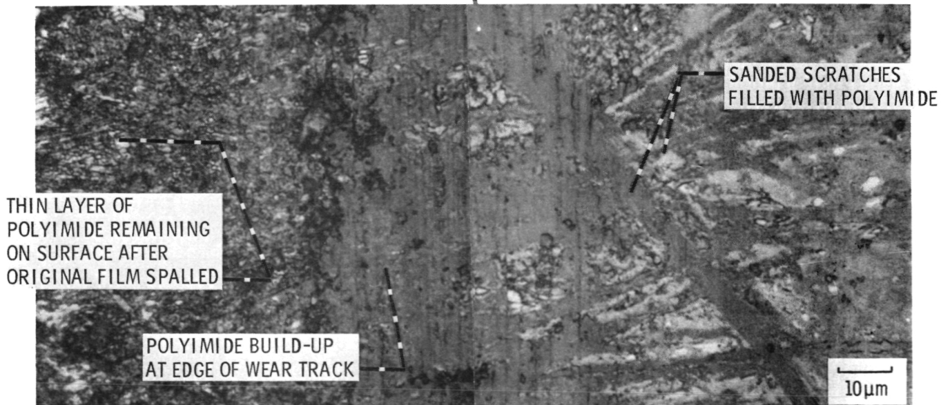
Figure 7. - Photomicrographs of the wear track (after 15 kilocycles of sliding) on a polyimide film which was thermally aged for 100 hours at 350°C before testing. The photomicrographs show the spallation of the film and the formation of a very thin secondary film on the metallic substrate (ref. 9).
