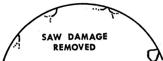
C. LAPPING, ETCHING AND POLISHING REMOVES SAW DAMAGE BUT NOT ALL OF THE GRINDING DAMAGE.
